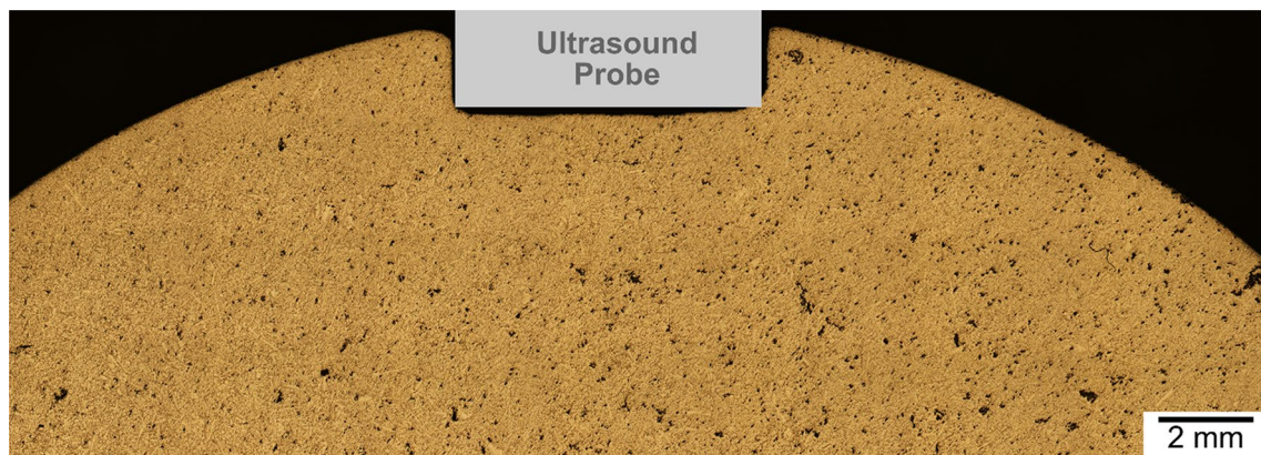
Figure 16 This image, stitched together from multiple optical micrographs, shows the dendritic microstructural morphology of the A356 control casting near the location of the ultrasound probe, which was inserted into the mold during casting but did not oscillate.
