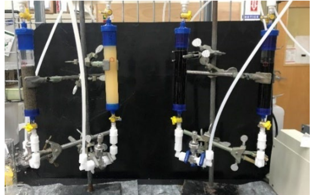
Column testing to support adsorbent media selection
