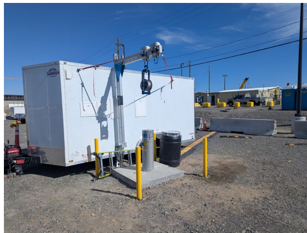
PNNL custom built field hydraulic testing trailer
