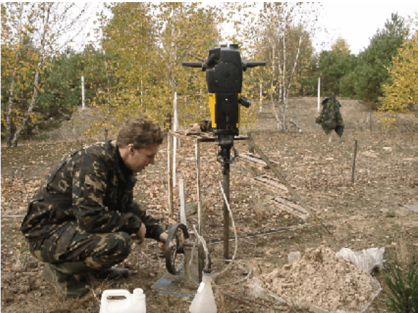
Field sampling using the push-drill system
