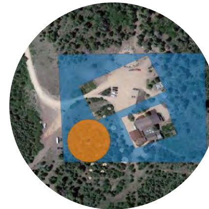
4. Biggest circle in remaining polygon determines maximum turbine size.
