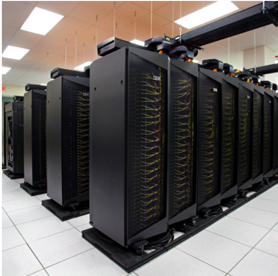
Carver @ NERSC.gov: 1202 compute nodes (9,984 processor cores)
