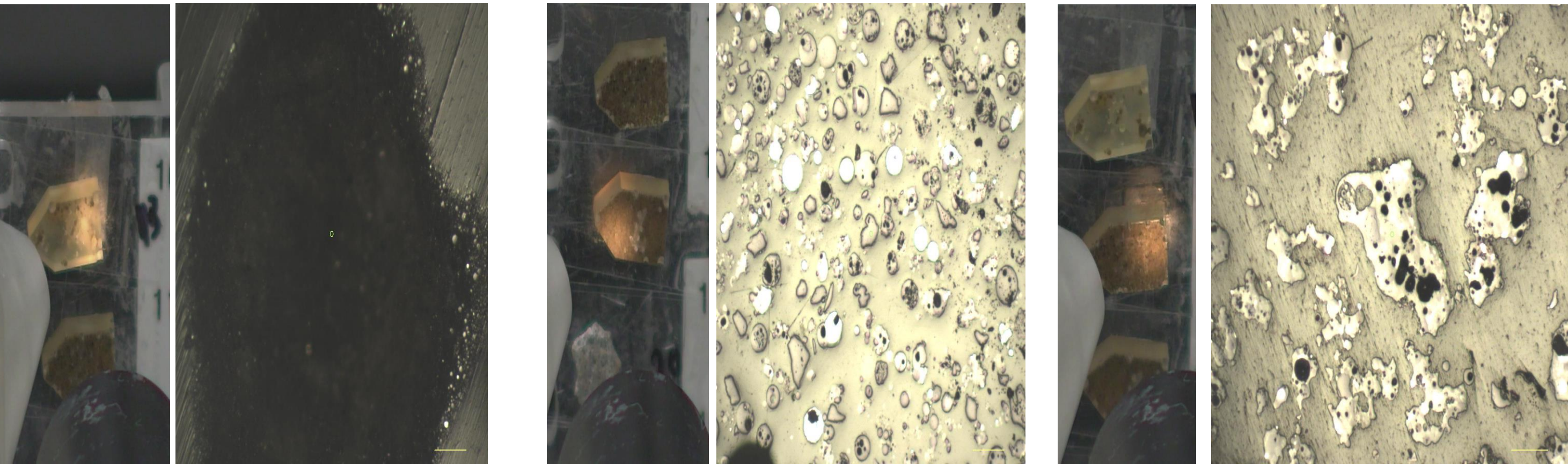
Fig 1: Raw fly ash in epoxy A) > 20 \mu\text{m} B) 53-75 \mu\text{m} C) 125-250 \mu\text{m}
