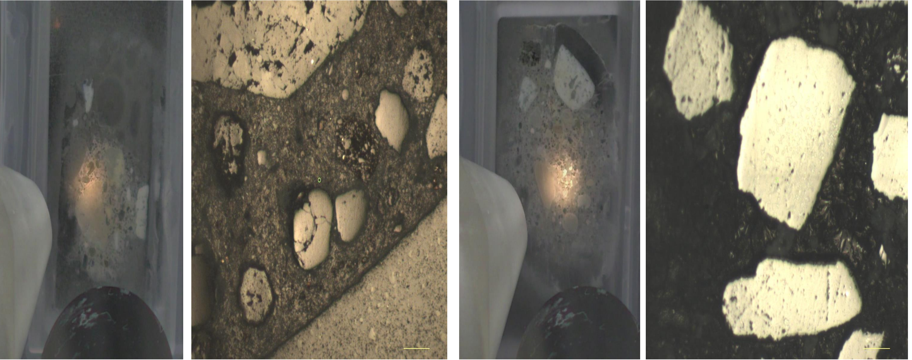
Fig 2: Concrete thin section A) 20% raw fly ash B)10% raw fly ash 10% beneficiated fly ash
