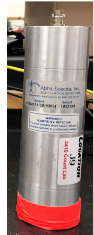
Alpha Spectra, Model 8TI040A1/2B (9266) Thin-Open Face Gamma Detector
