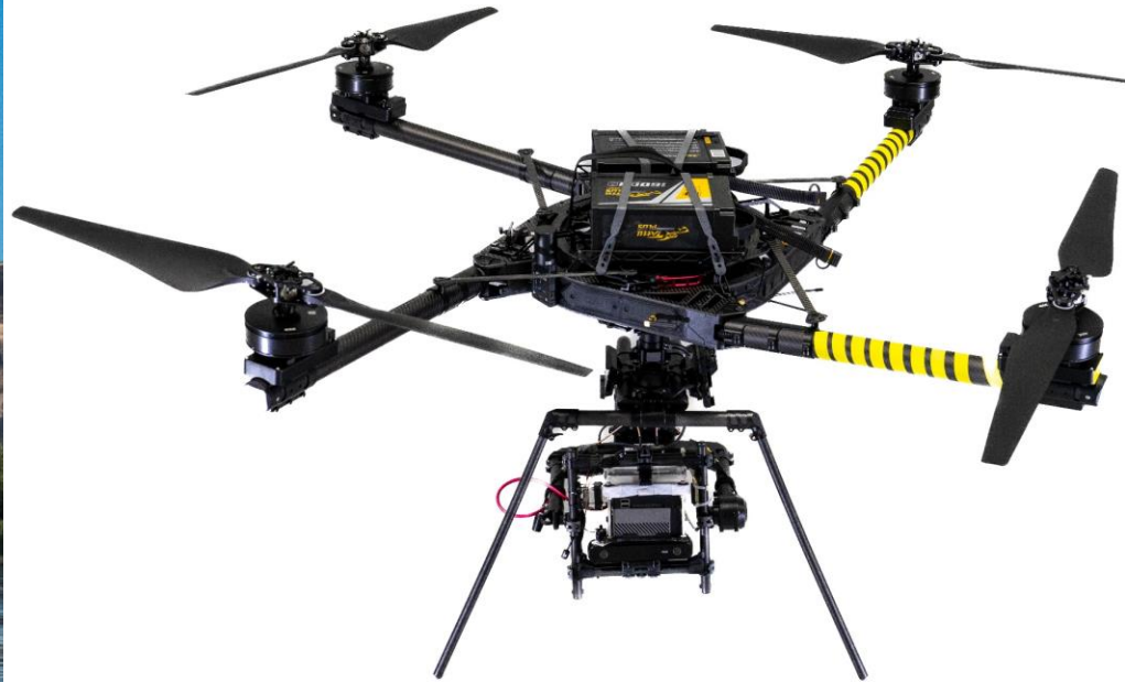
Freefly Alta X Maximum Take-Off Weight (MTOW): 76.9 lbs
