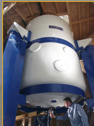
900-MHz NMR spectrometer allows scientists to transcend previous limits in catalyst characterization.
