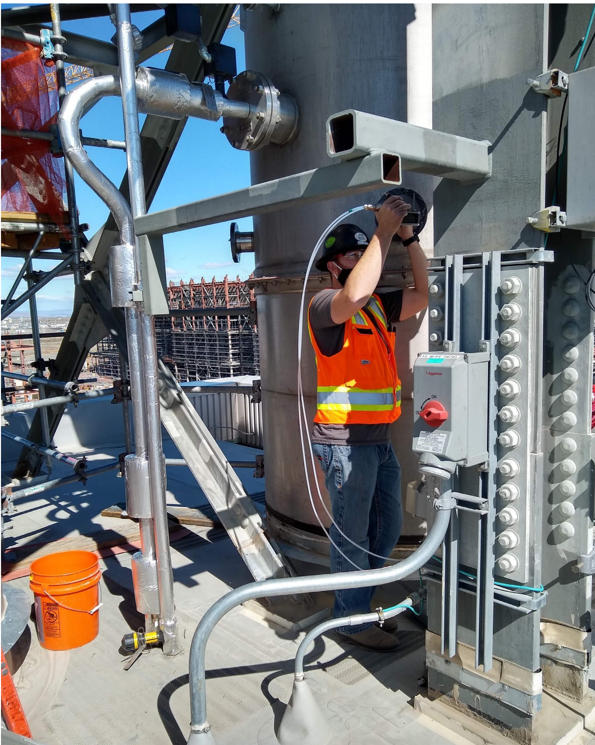
Figure 5. LAW LV-C2 Stack on the Facility Rooftop. Bison staff member is measuring flow angle at the east port, and the west port is visible behind him.
