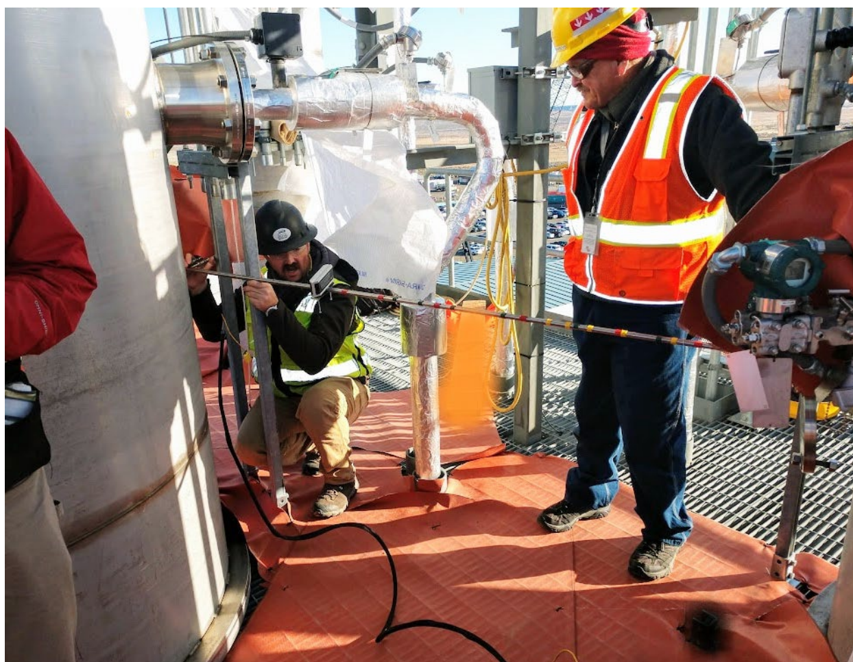
Figure 2. Flow Angle Testing on the LB-C2 Stack, with Probe Maneuvered around the LB-S1 Pitot Support
