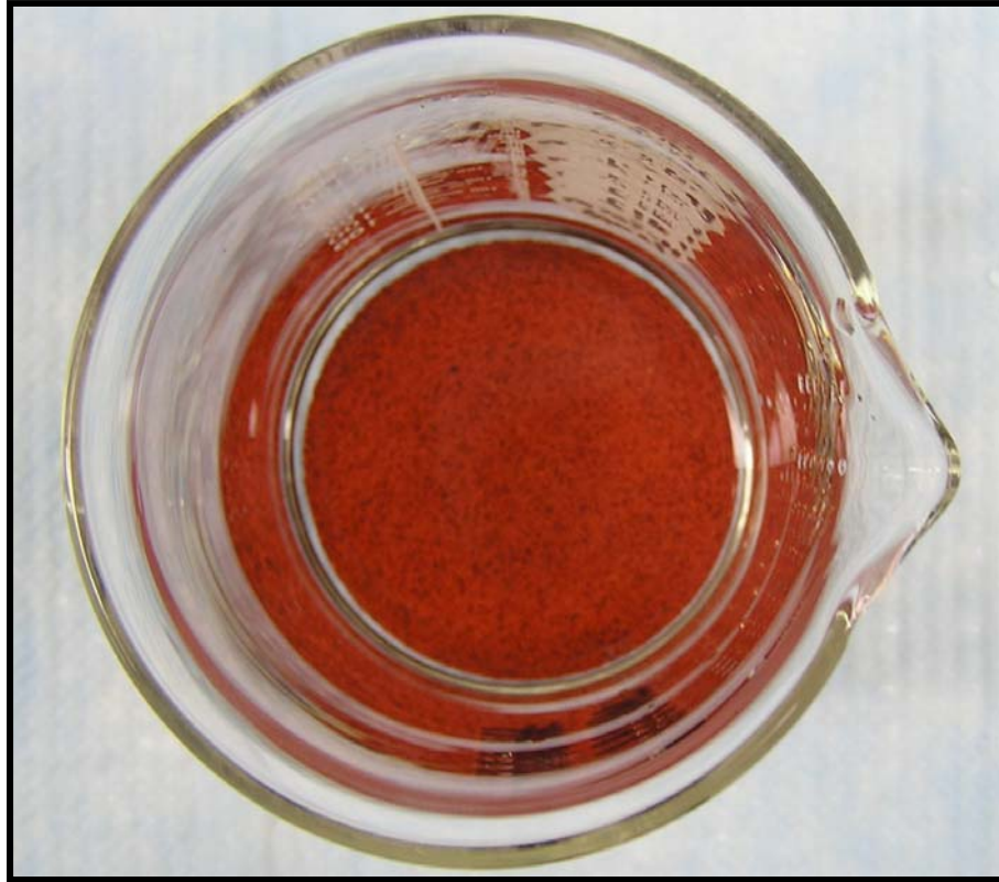
Figure 3.1. Representative SRF Resin Sample for Column Testing Showing Darkened Resin Beads
