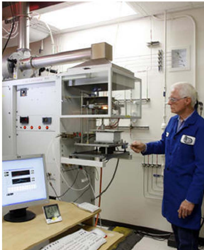
Figure 3.3. Cone Calorimeter Apparatus at SwRI
