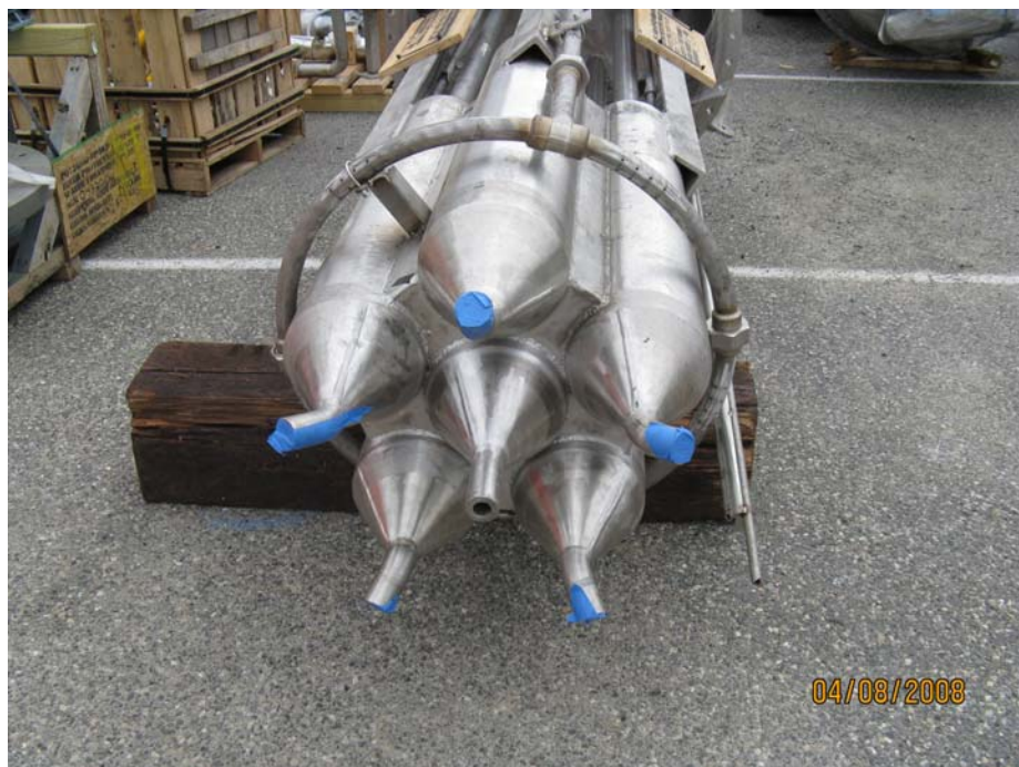
Figure 4.16. Delivered PJMs Before Installation into Tank T02A
