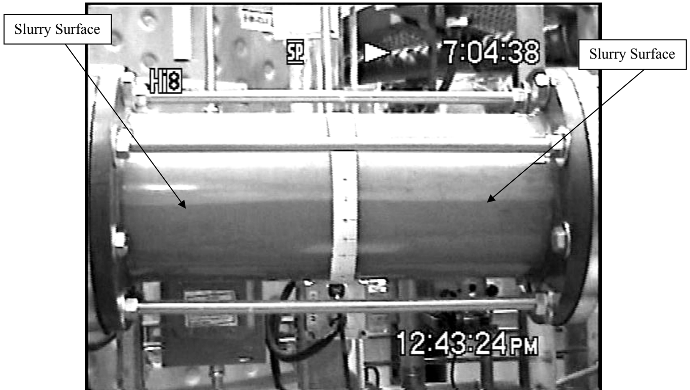
Figure A.62. Upstream, Slope = 1:50, Velocity = 2.0 ft/s
