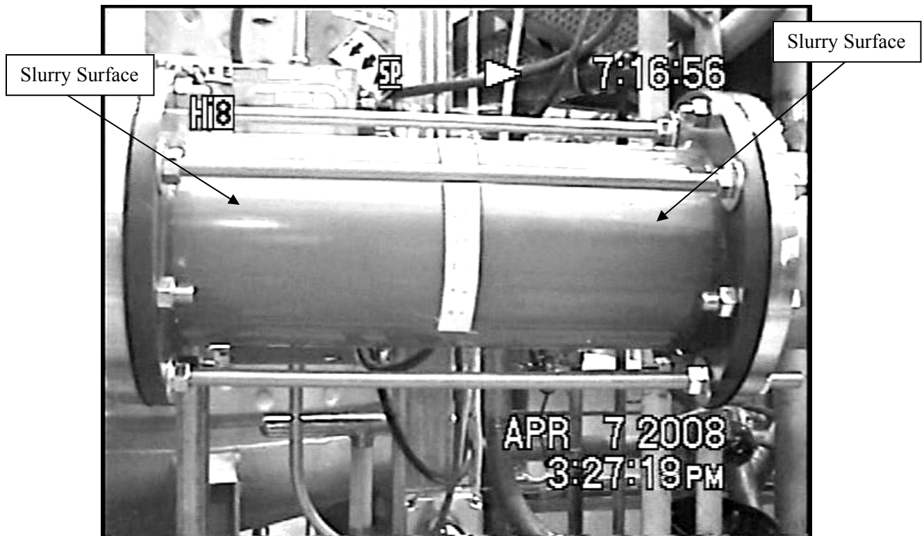
Figure A.13. Upstream, Slope = 1:125, Velocity = 5.0 ft/s
