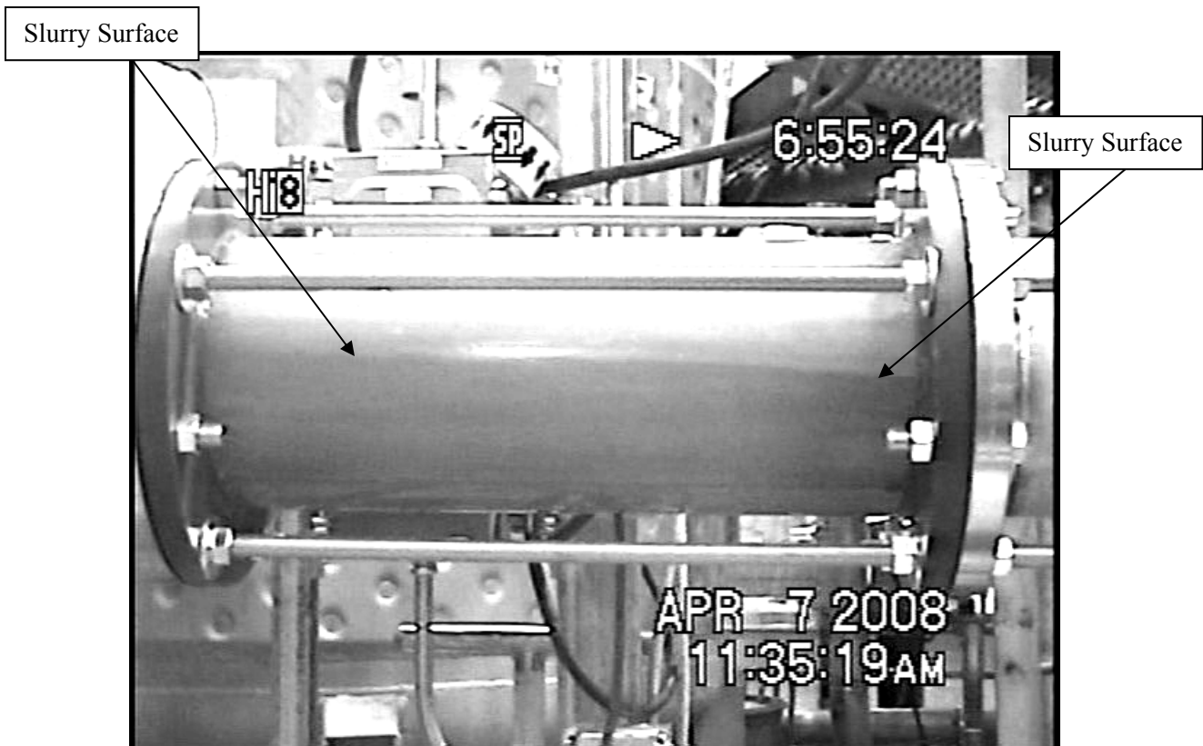
Figure A.5. Upstream, Slope = 1:125, Velocity = 7.0 ft/s
