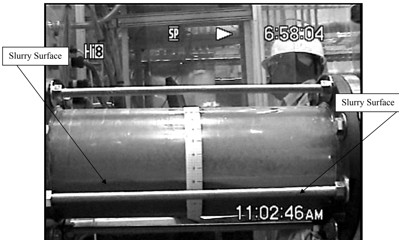
Figure A.52. Downstream, Slope = 1:50, Velocity = 5.0 ft/s
