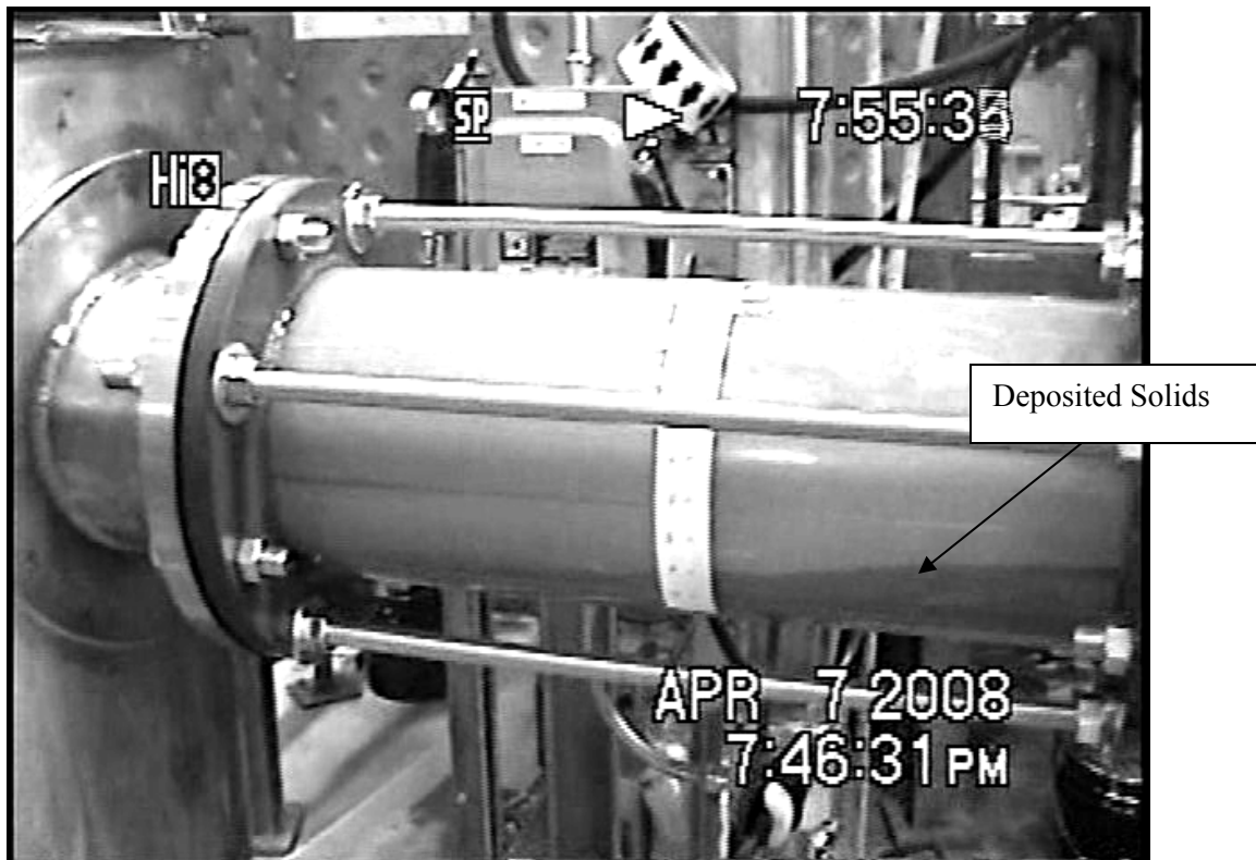
Figure 8.8. Upstream Post-Test Deposition
