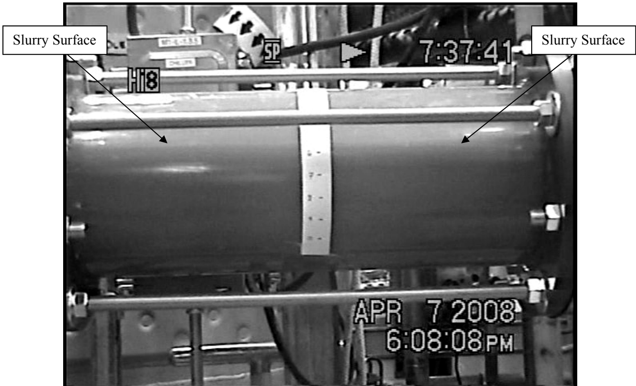
Figure 8.3. Side View of Upstream Transparent (Clear) Section with Measuring Tape
