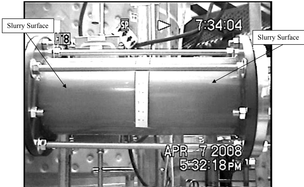
Figure A.19. Upstream, Slope = 1:125, Velocity = 3.5 ft/s
