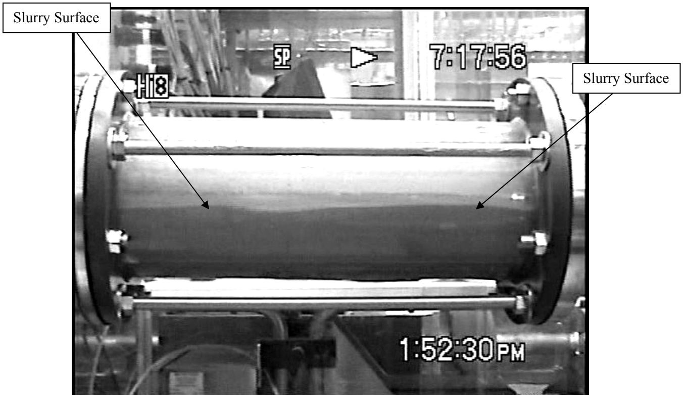
Figure A.12. Downstream, Slope = 1:125, Velocity = 5.5 ft/s
