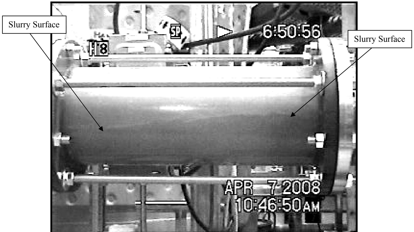
Figure A.3. Upstream, Slope = 1:125, Velocity = 7.5 ft/s
