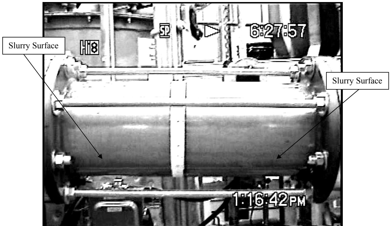
Figure A.41. Upstream, Slope = 1:20, Velocity = 2.0 ft/s
