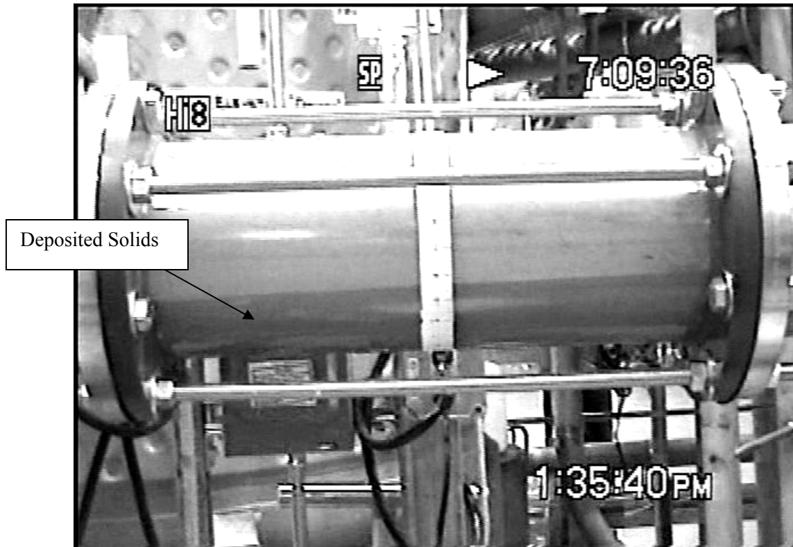
Figure 8.15. Upstream, Slope = 1:50, Post-Test Deposition
