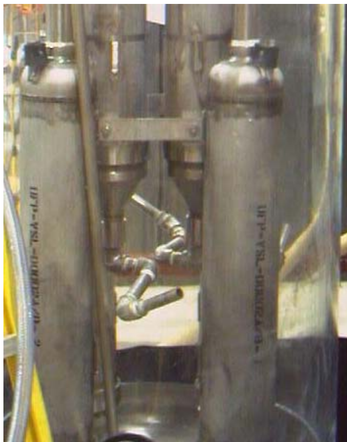
Figure 7.9. UFP Rams-Head Discharge Nozzles for the All-in Configuration
