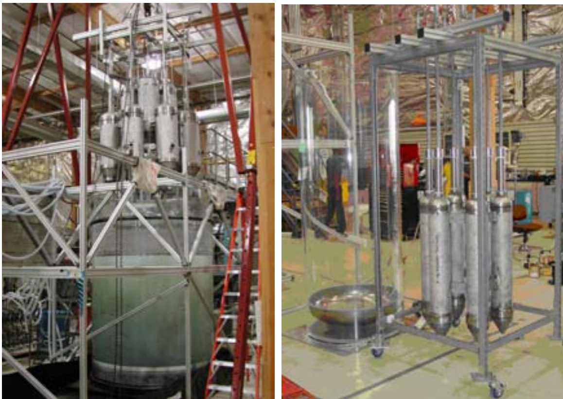
Figure 5.7. LS Scaled Prototype Vessel with PJM Configuration Lifted into Test Vessel (left) and UFP Scaled Prototype Vessel with PJM Configuration Removed for Reconfiguration (right)
