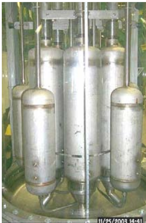
Figure 8.12. Final CRV Test Configuration; 8-inch Diameter Cluster PJM and Charge Vessel Assembly (1.5-inch-diameter nozzles installed)
