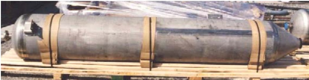
Figure 5.4. A Pulse Tube Before Installation in the Large-Tank Test System. The pulse tubes were connected to 2-inch pipe couplings that enabled insertion of level gauges and attachment of the air/vacuum lines required for PJM operation.
