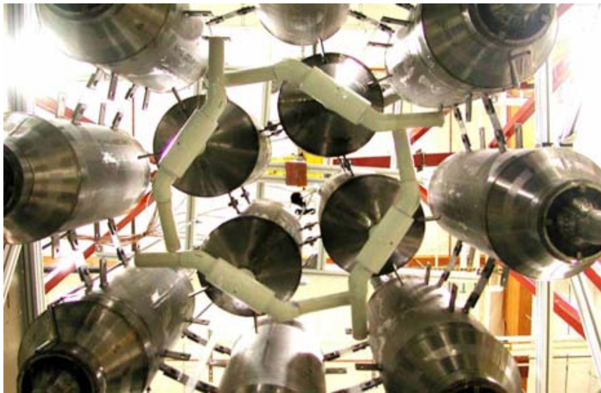
Figure 7.7. LS All-in Nozzle Configuration (from below)
