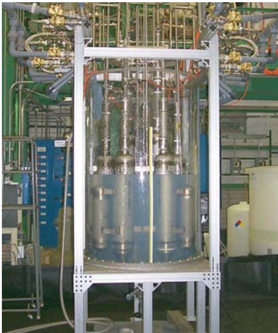
Figure 5.9. Scaled CRV Test Stand (baseline PJM configuration installed)
