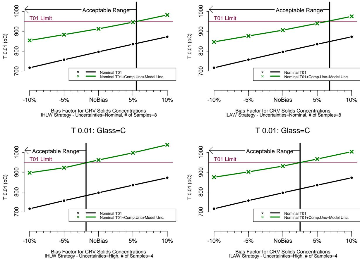
**Figure 6.3.  $T_{0.01}$  Nominal and 90% UCCI Results as a Function of HLW CRV Mixing/Sampling Bias. The acceptable range of bias for each situation is marked with an arrow.**
