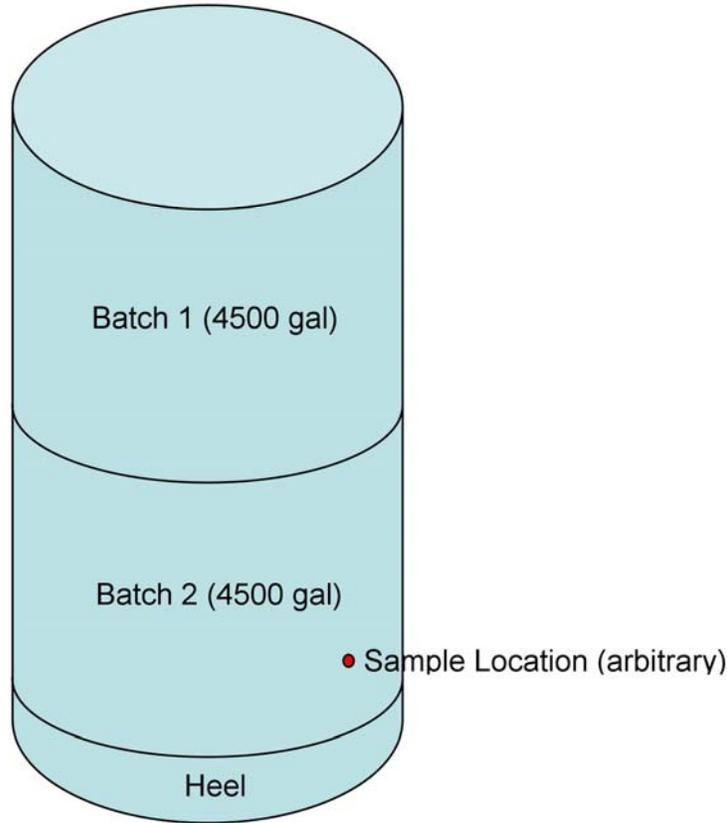
**Figure 8.2. Illustration of HLW CRV and Two Batches for Transfer to the MFPV**
