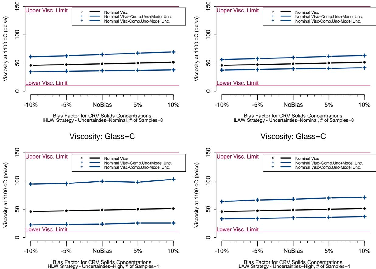
**Figure 6.6. Viscosity at 1100°C Nominal and Two-Sided 90% CCI Results as Functions of HLW CRV Mixing/Sampling Bias**
