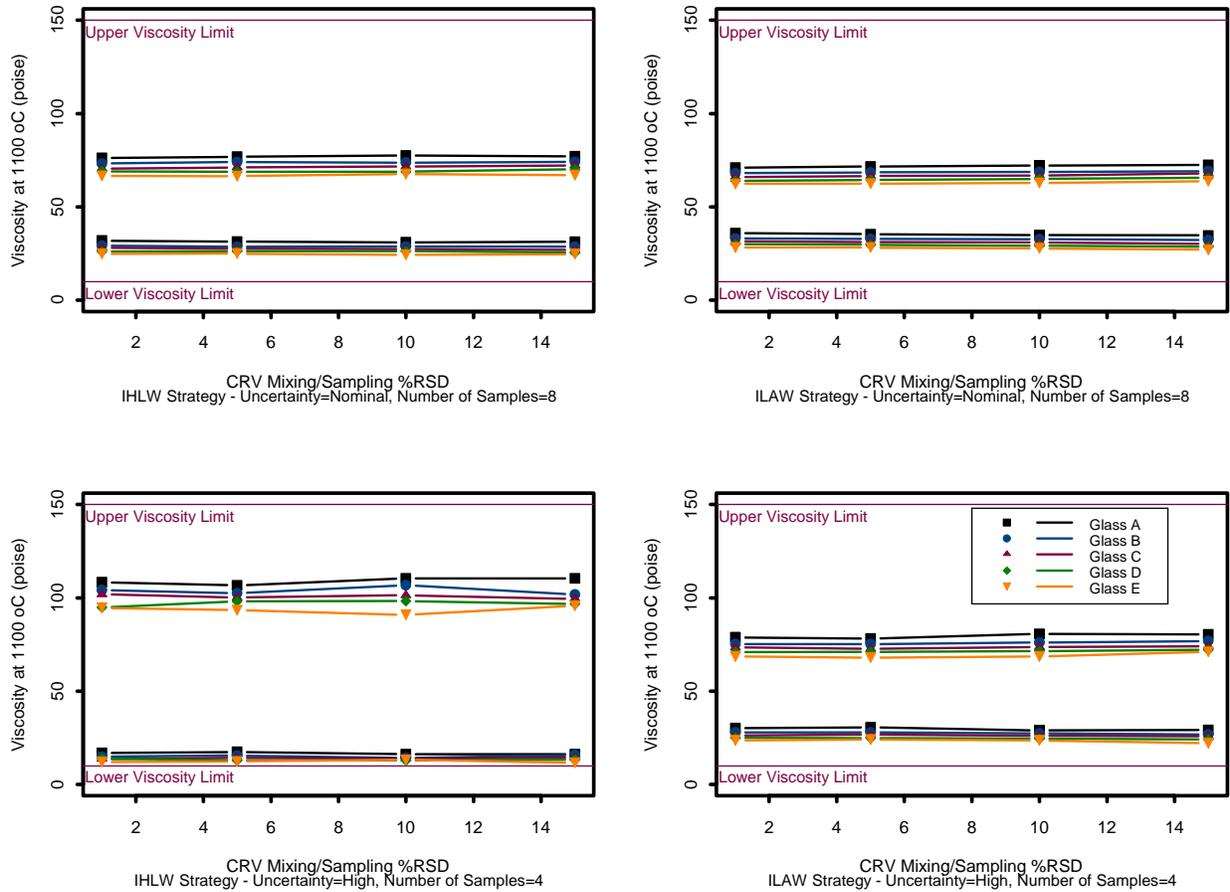
**Figure 5.6. Viscosity at 1100°C Plots Showing Two-Sided 90% CCI as Functions of HLW CRV Mixing/Sampling Random Uncertainty %RSD for Each Glass Formulation**
