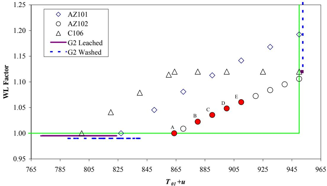
**Figure 2.1. Plot of WL Factor Versus  $T_{0.01} + u$  for Three Actual Waste Compositions and G2 Output Compositions Leached and Washed**
