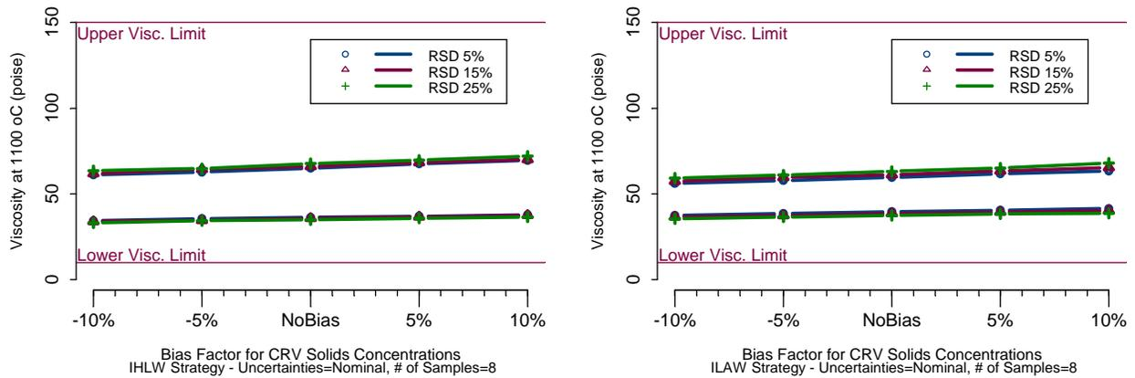
**Figure 7.5. Viscosity at 1100°C Two-Sided 90% CCI Results as Functions of HLW CRV Mixing/Sampling Bias and Random Uncertainty**
