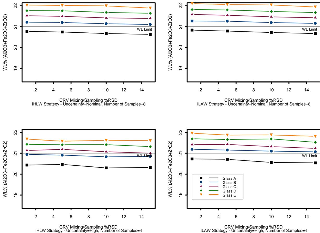
**Figure 5.4. Waste-Loading Plots Showing 90% LCIs as a Function of HLW CRV Mixing/Sampling Random Uncertainty %RSD for Each Glass Formulation**
