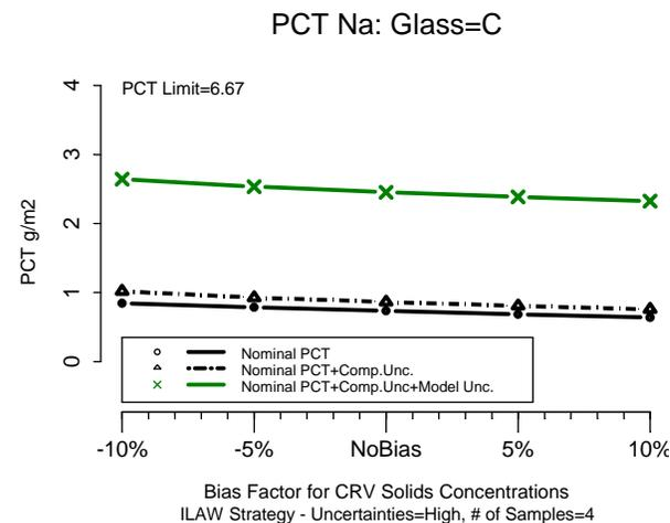
**Figure 6.1. PCT Nominal and 90% UCCI Results as a Function of HLW CRV Mixing/Sampling Bias**
