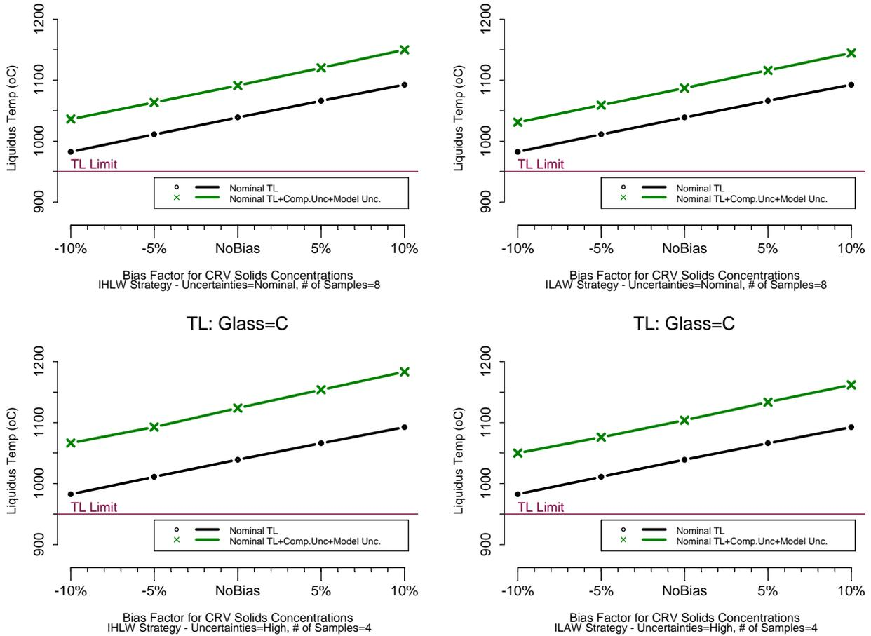
**Figure 6.2.  $T_L$  Nominal and 90% UCCI Results as a Function of HLW CRV Mixing/Sampling Bias**
