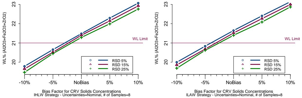
**Figure 7.3. Waste Loading 90% LCI Results as Functions of HLW CRV Mixing/Sampling Bias and Random Uncertainty**
