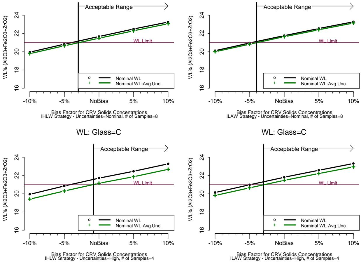
**Figure 6.4. Waste Loading Nominal and 90% LCI Results as a Function of HLW CRV Mixing/Sampling Bias. The acceptable range of bias for each situation is marked with an arrow.**
