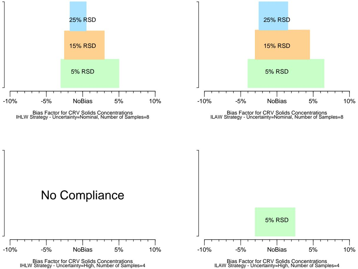
**Figure S.1. Ranges of CRV Mixing/Sampling Bias that Allow Compliance and Processing Properties to be Satisfied with 90% Confidence. The dependence of the ranges on CRV mixing/sampling random uncertainty %RSD is shown.**
