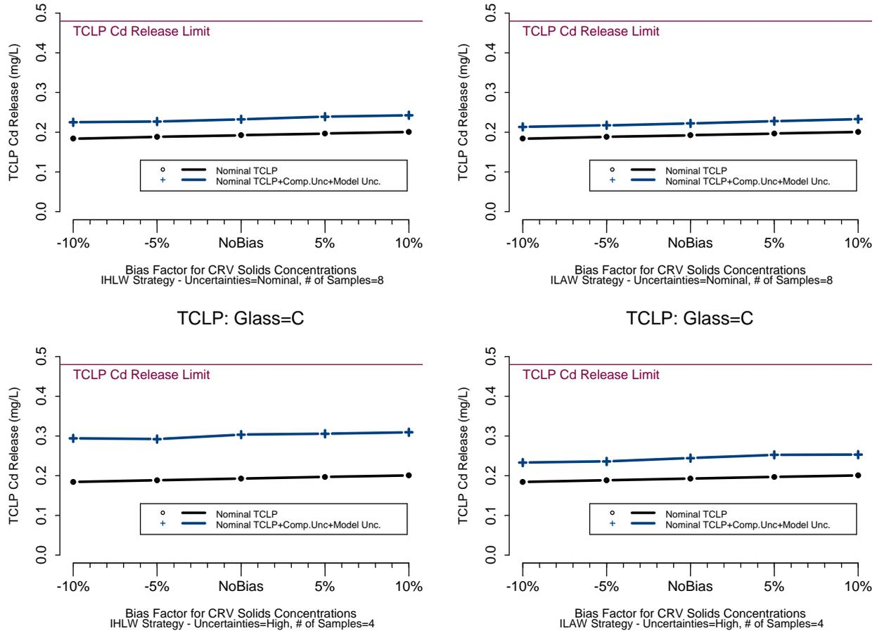
**Figure 6.5. TCLP Cd Release Nominal and 90% UCCI Results as a Function of HLW CRV Mixing/Sampling Bias**
