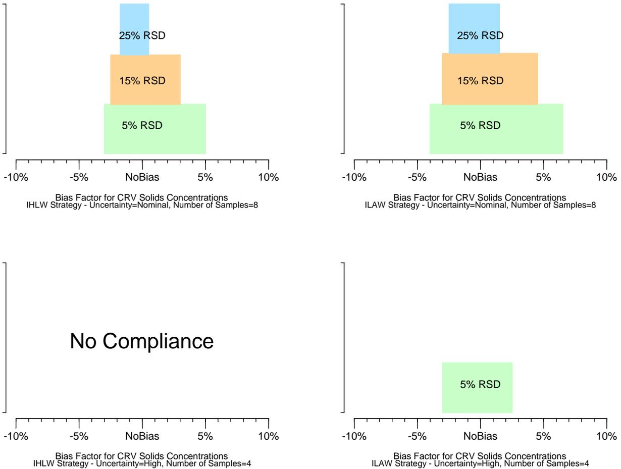
**Figure 8.1. Ranges of HLW CRV Mixing/Sampling Bias that Allow Compliance and Processing Properties to be Satisfied with 90% Confidence. The dependence of the ranges on HLW CRV mixing/sampling random uncertainty %RSD is shown.**
