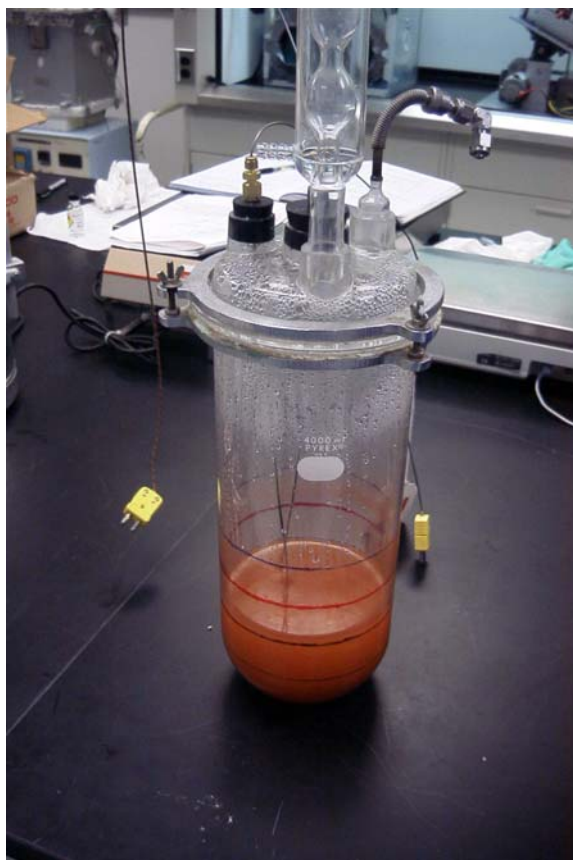
Evaporator Concentrate at the Conclusion of the pH = 8.4 Test
