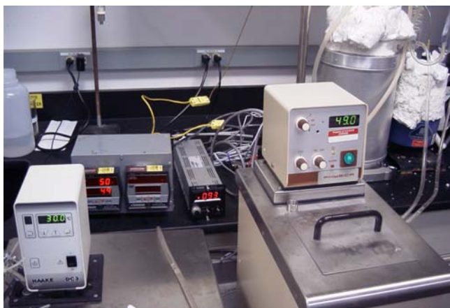
Column Temperature Control Recirculators, Foreground; Boiler Temperature Controller, Inleakage Flow Controller, Background
