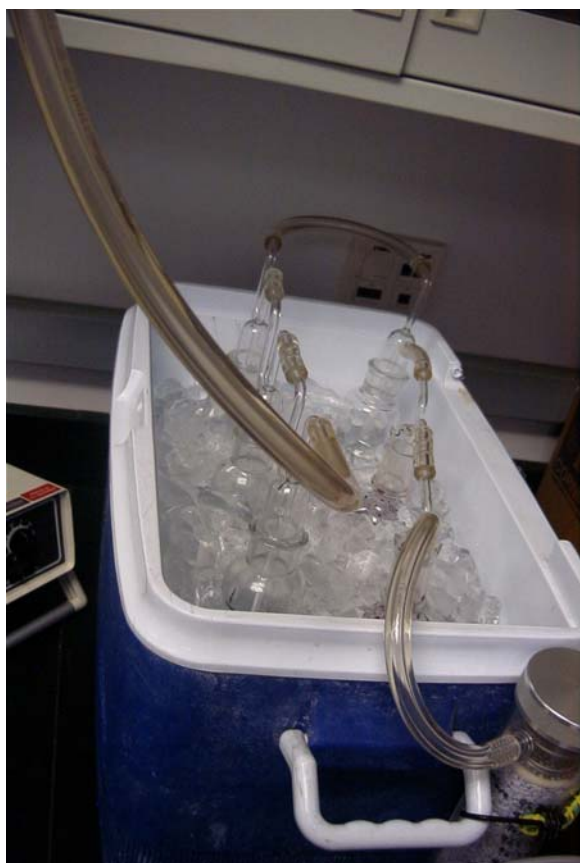
Mercury Vapor Chemical Scrubbers
