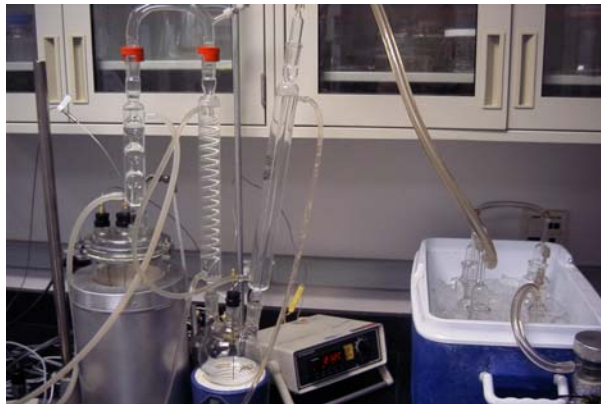
Boiler, Distillation Columns, Condensate Pot, and Gas Scrubbers
