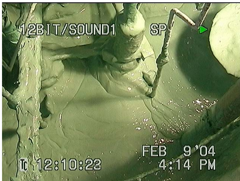
Figure 5.8. Example of Simulant Cake out and Uneven Surface (LS Sequence 15A)
