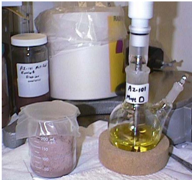
a) GFC (LAWB-83) and 2.75 M Na AZ-101 Envelope B pretreated LAW mixing/aging sample before mixing
