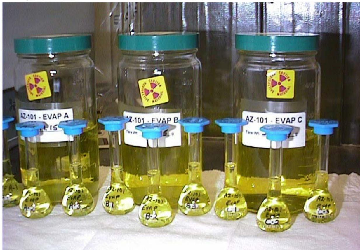
Figure 2.1. Photograph of  $1.75$ ,  $2.75$ , and  $3.75 \text{ M}$  Na AZ-101 Pretreated Wastes
