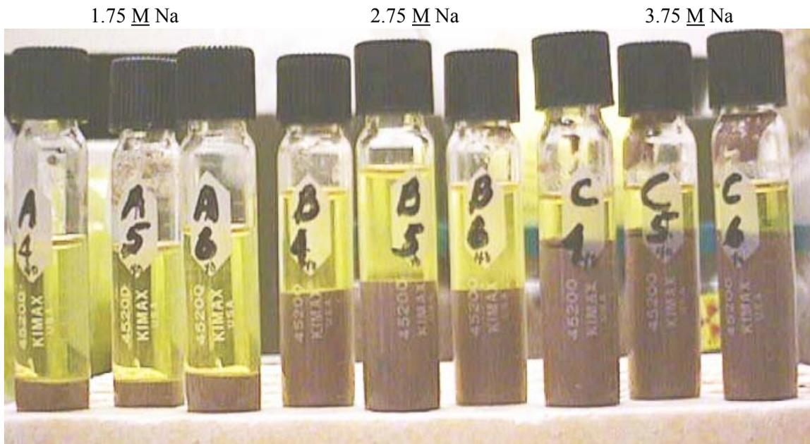
Figure 3.1. Photograph of AZ-101 Envelope B Melter Feed Physical-Property Samples
