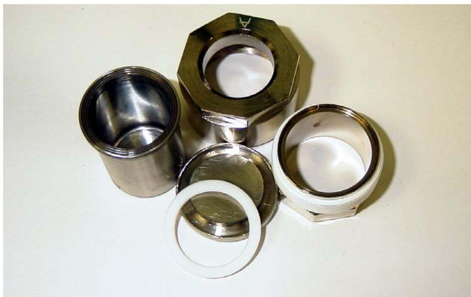
**Figure 5.3. Desensitized Type 304L Stainless Steel, 22 mL, PCT Vessel and Lid (Teflon gasket, nickel-plated brass compression fittings are also shown)**
