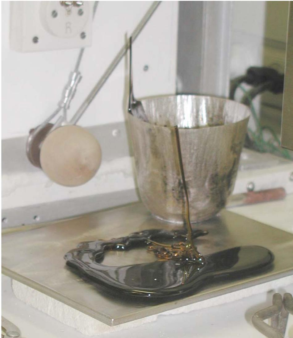
**Figure 6.1. Freshly Poured AP-101Glass Quenched on the Stainless Steel Plate**
