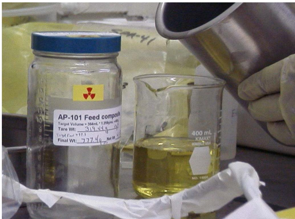
**Figure 5.1. AP-101 Pretreated Waste before Adding Glass Former Chemicals (shown in a 400-mL glass beaker; waste solution was originally stored in the 0.5-L container on the left)**
