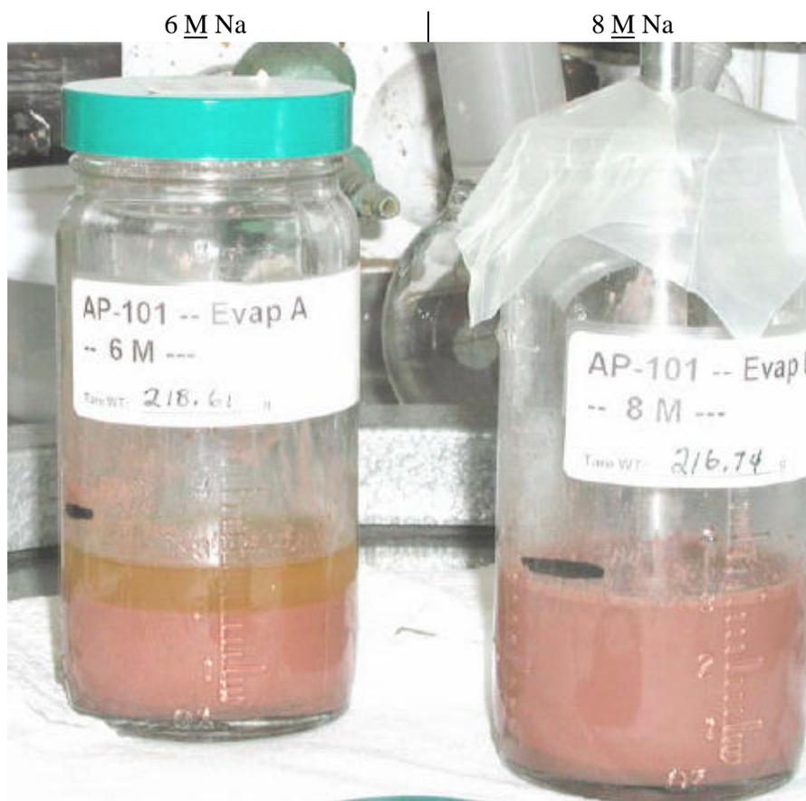
**Figure 2.3. AP-101 Melter Feed Samples Following Glass Former Chemical Additions**
