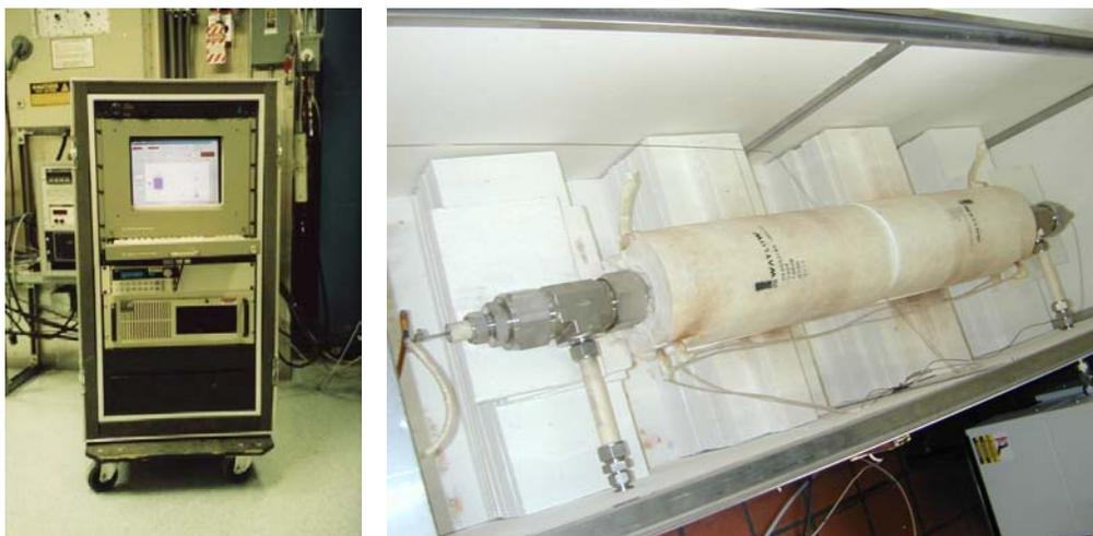
**Figure 5. Components for the Field Corona System. Left – Control Station and Power Supply. Right – Cylindrical Packed-Bed Corona Reactor with Inlet, Outlet, and Electrical Connections.**
