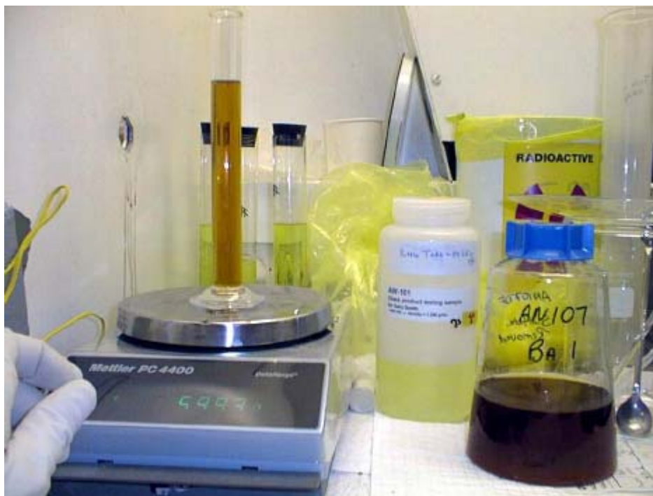
Figure 3.1. Density Measurement of AN-107 Pretreated Waste Prior to Feed Preparation. AW-101 Pretreated Waste is in Plastic 1L Container in Center of Picture.
