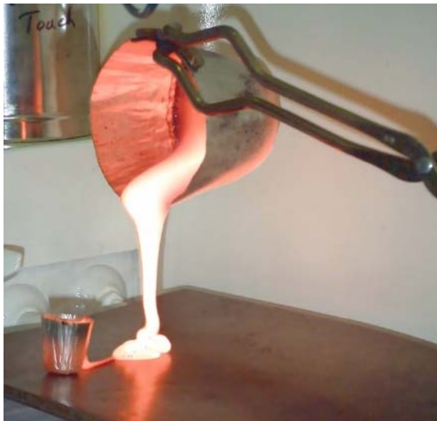
Figure 4.6. The AN-107 Glass in The Process of the Final Pour Onto the Stainless Steel Pour Plate. The 20 ml Crucible for the Canister Centerline Cooling Heat Treatment is Red Hot with Freshly Poured Glass.
