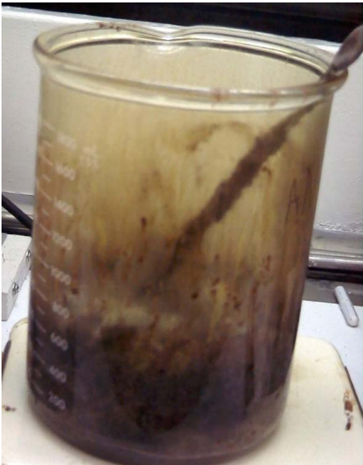
Figure 4.5. AN-107 Feed During Exothermic Reaction. Note the Drainage of Material that Adhered to Beaker Wall and the Cloudy, Frosted Appearance of the Beaker From Condensate During Reaction.
