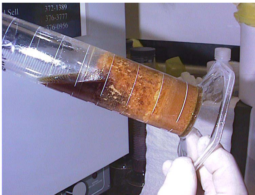
Figure 2.3. Close Up of Solids Precipitated Out of 10M AN-107 Sample. While Loosely Packed, Solids Account for Roughly 70% of the Sample Volume
