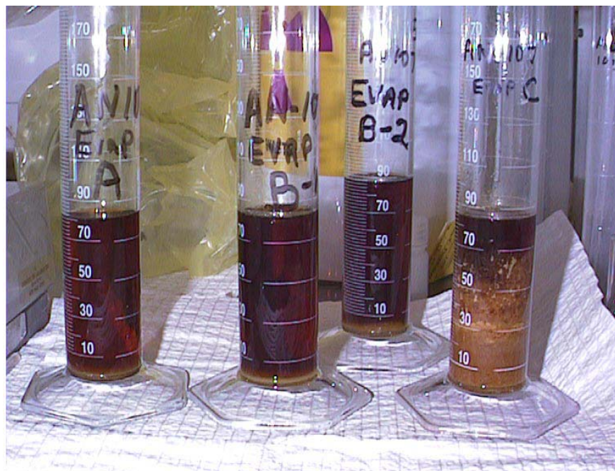
Figure 2.2. AN-107 Samples Following 24 hours at 50°C. This Photograph Was Taken Two Weeks After Completion of Evaporation. Note Solids in Sample C That Were Not Observed 2 Days Prior to This Photograph. Samples A, B (B-1 and B-2), and C are 6M, 8M, and 10M Sodium Respectively
