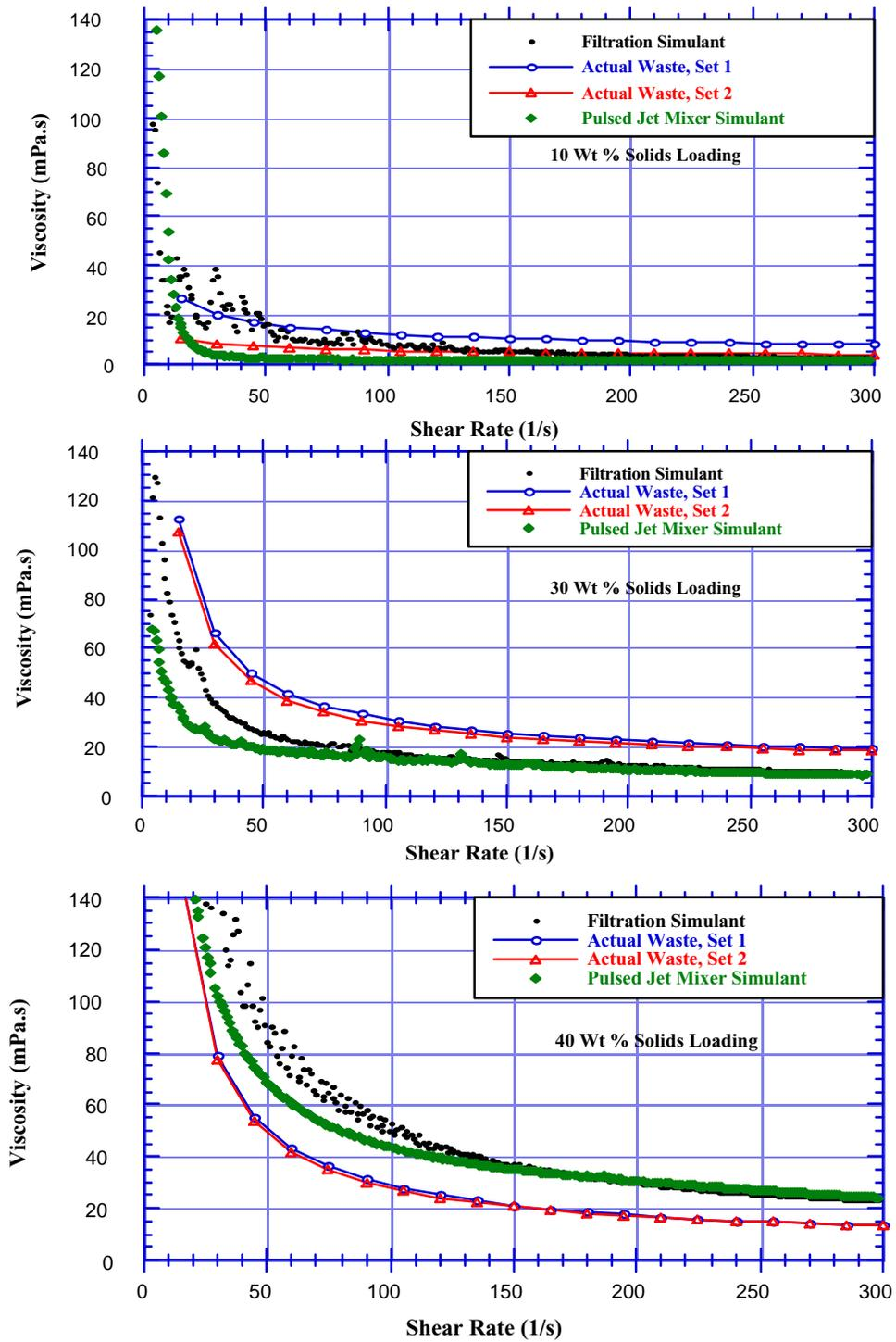
Figure A.1. Comparison of the Viscosity v. Shear Rate behavior for the Pulsed Jet and CUF Simulants with that of the Actual Waste.
