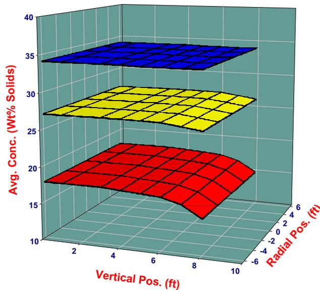
Figure 3.1. Mixer Performance at Different Initial Solids Loading of 17 (Red), 28 (Yellow), and 36-wt% (Blue) when All Four-Pulse Tubes Are Operated At Maximum Frequency.
