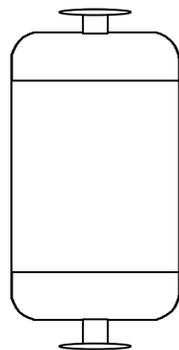
Figure 2.5. Schematic of the RFD Charge Vessel.
