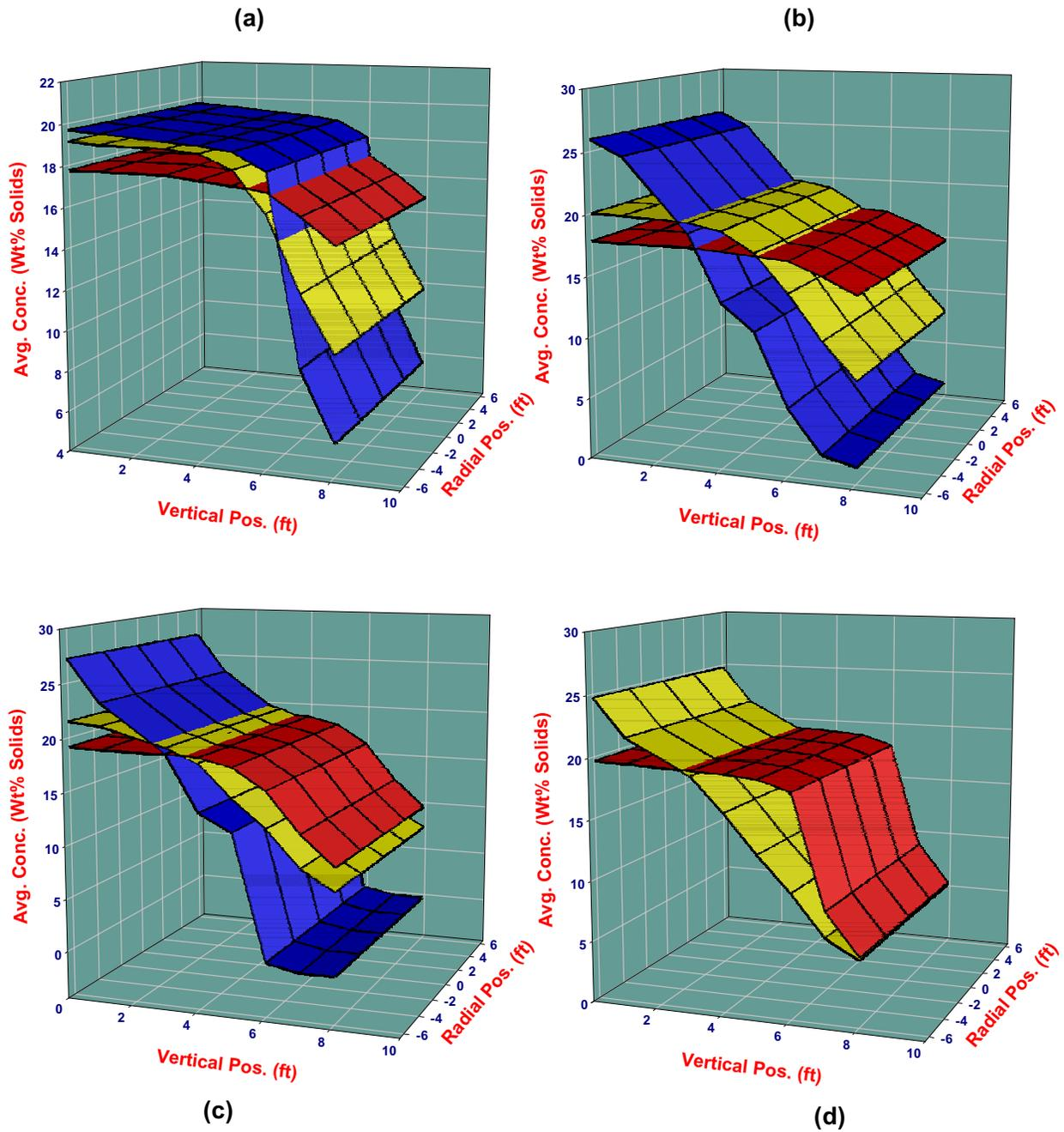
Figure 3.6. Mixing Profiles at 17-wt% Initial Solids Loading. (a) Four (Red) and Two (Yellow) PJM Operating at Maximum Frequency of Operation. (b) Four PJM's Operating at 100 (Red), 50 (Yellow), and 10% (Blue) of Maximum Frequency. (c) Two PJM's Operating at 100 (Red), 50 (Yellow), and 10% (Blue) of Maximum Frequency. (d) One PJM Operating at 100 (Red), and 50% (Yellow) of Maximum Frequency.
