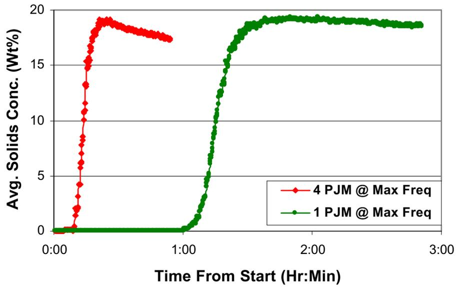
Figure 3.3. Average Solids Concentration Profiles at 17-wt% Initial Solids Loading.
