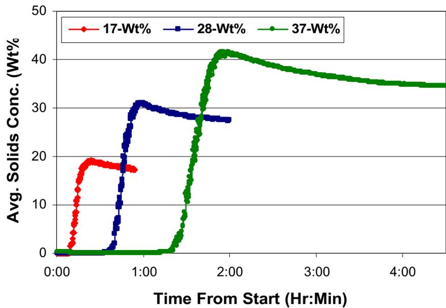
Figure 3.4. Average Solids Concentration Profiles at 17, 28, and 36-wt% Initial Solids Loading.
