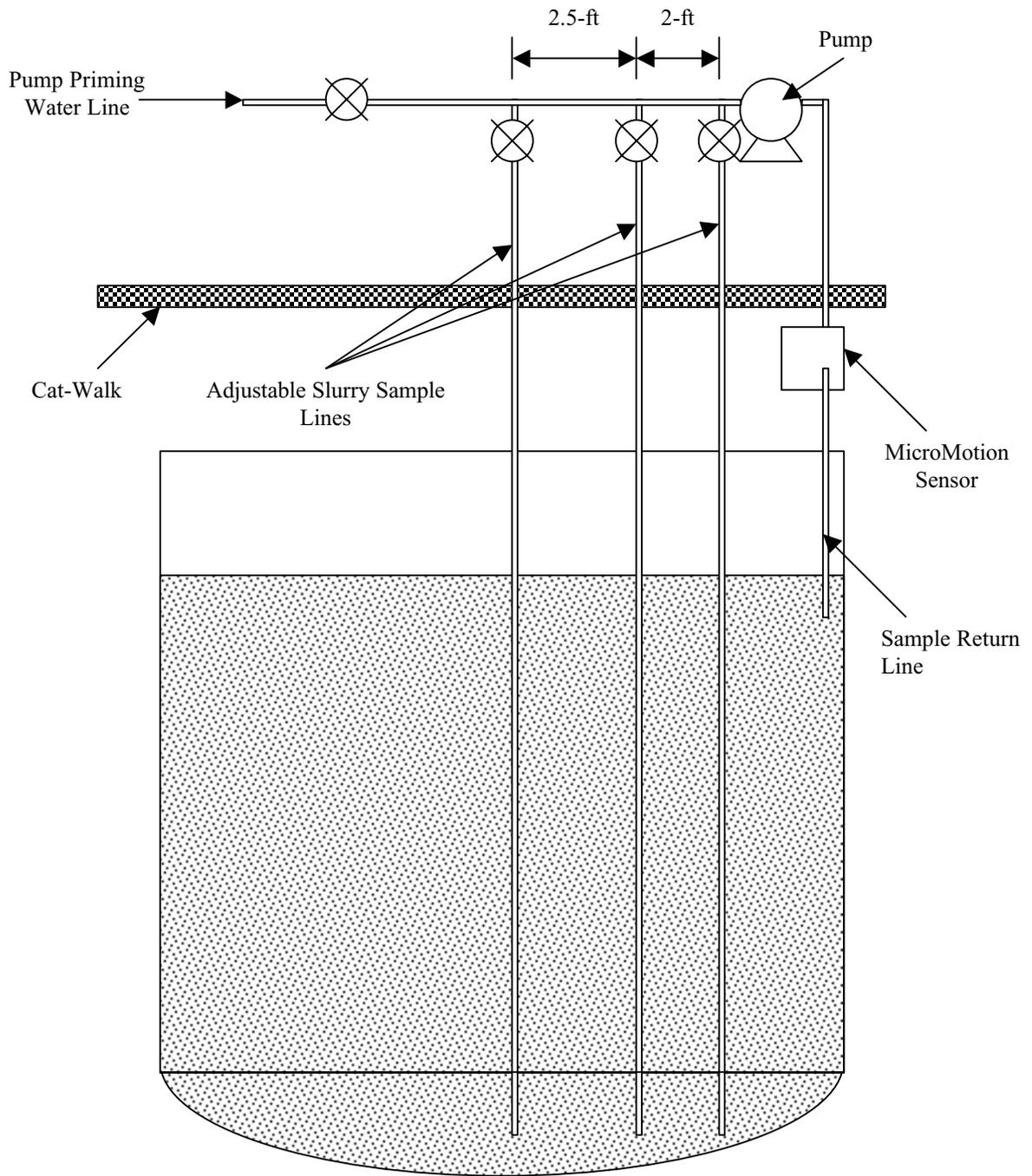
Figure 2.8. Schematic of the Sampling Arrangement Used to Measure the Slurry Concentration within the Tank.
