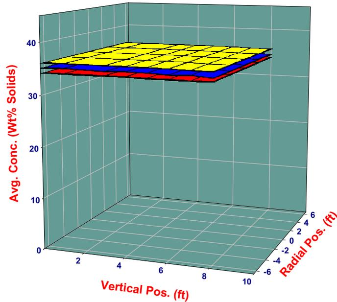
Figure 3.8. Mixing Profiles for 36-Wt% Initial Solids Loading. Curves in Red and Yellow are for 4 and 1 PJM Operated at Maximum Frequency. Blue Curve Represents the Data for 4 PJM at 50% Frequency.
