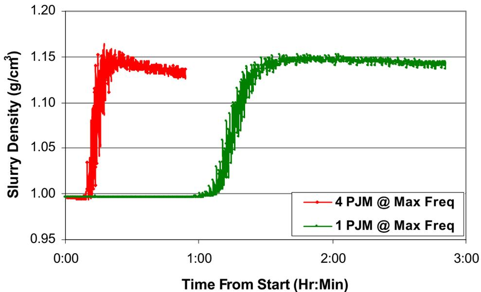
Figure 3.2. Slurry Density Profiles at an Initial Solids Loading of 17-wt%.
