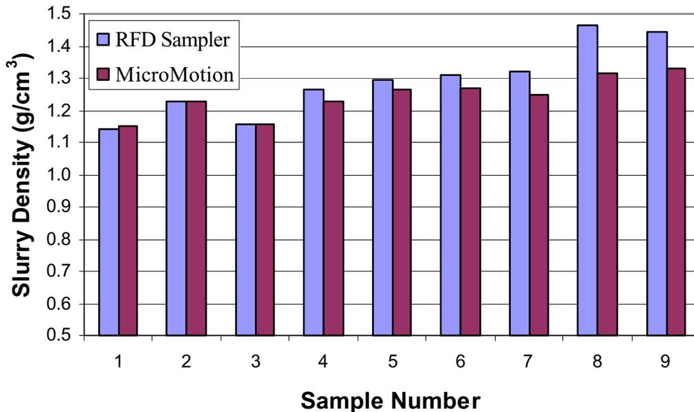
Figure 3.5. Comparison of RFD Sample Density with that Obtained from the MicroMotion Density Meter Sample Drawn at the Same Location.
