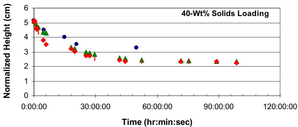
Figure A.2. Comparison of the Settling Rate Behavior of the Pulsed Jet Simulant (in green) with that of the CUF Simulant (in Red) and the Actual Waste (in Blue).
