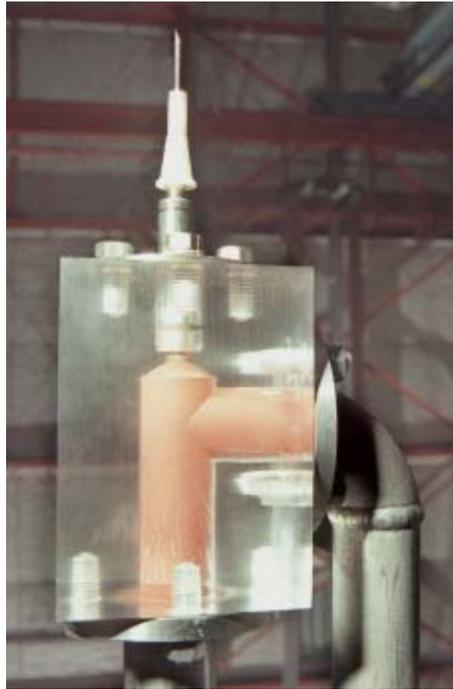
Figure 2.4. Photograph of the RFD Sampling Tee.
