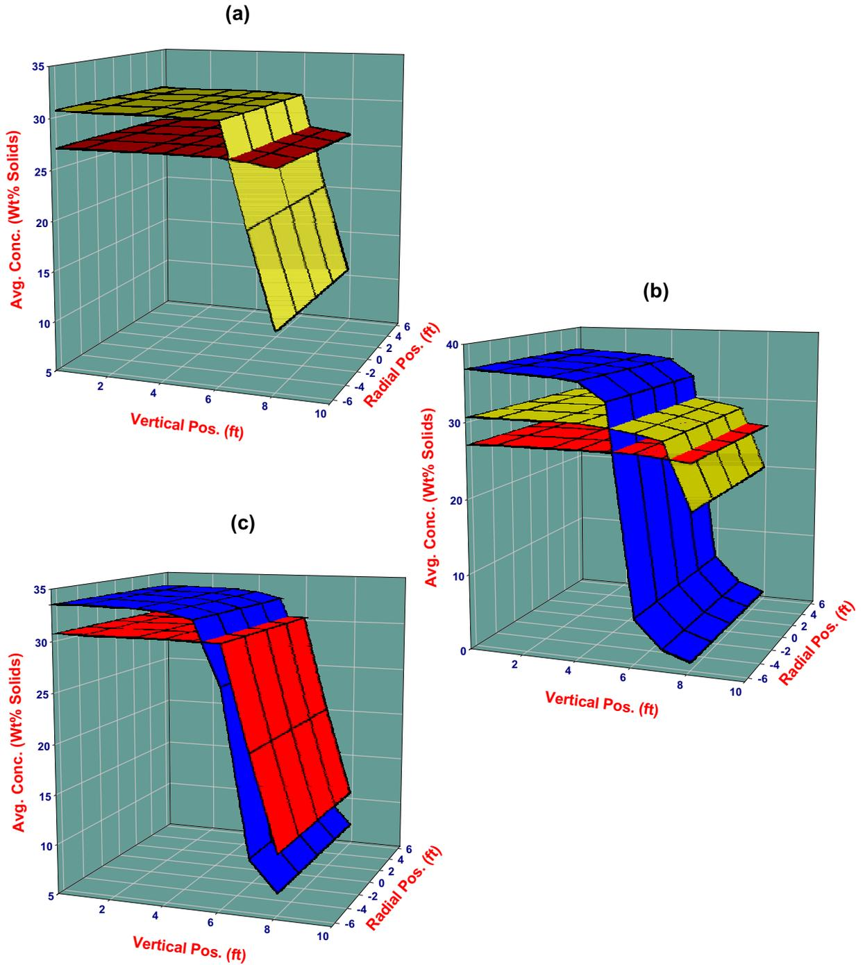
Figure 3.7. Mixing Profiles at 28-wt% Initial Solids Loading. (a) Four (Red), and One (Blue) PJM Operating at Maximum Frequency of Operation. (b) Four PJM's Operating at 100 (Red), 50 (Yellow), and 10% (Blue) of Maximum Frequency. (c) Two PJM's Operating at 100 (Red), 50 (blue) of Maximum Frequency.
