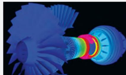
In 2006, PNNL and Advanced Virtual Engine Test Cell Inc. set out to improve computer models that simulate turbine engine performance and could reduce manufacture time. This simulation of a full aircraft jet engine includes all major components. Color indicates pressure changes in the engine and temperature changes in the combustor.
