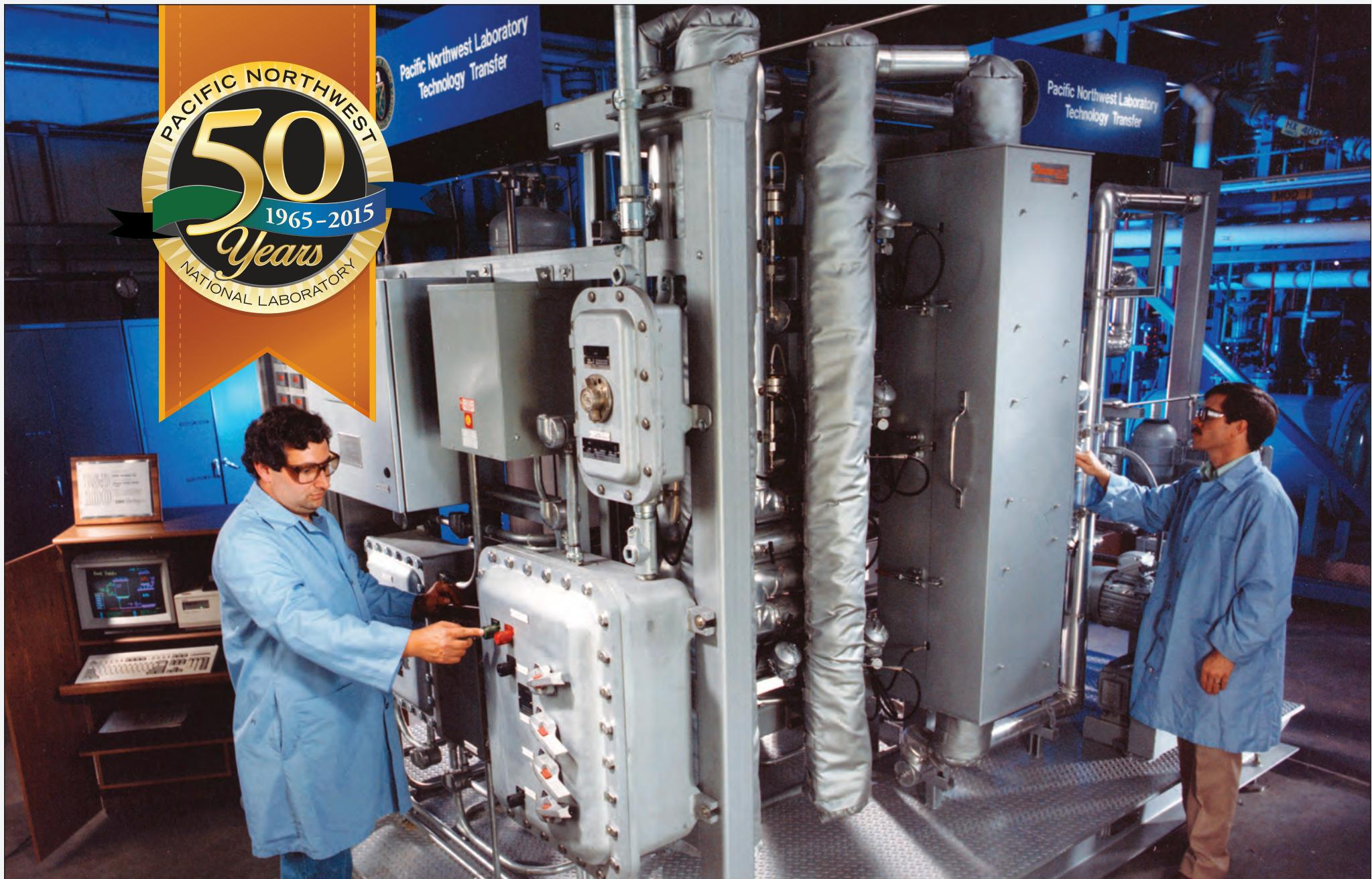
In the 1990s, PNNL researchers used this equipment to explore and advance the use of hydrothermal processing to convert wet biomass streams into fuel gas. Today, this equipment is at the site of a Florida-based industrial partner that will use it to convert algae to biocrude oil. PNNL researchers will help with the startup of the equipment in support of the effort.
