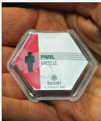
This palm-sized detector is used by medical radiology technicians, cancer treatment specialists and others to measure the radiation they receive at the workplace. The technology was developed at PNNL and commercialized by Battelle and Landauer, the world leader in providing personnel radiation monitoring services.
