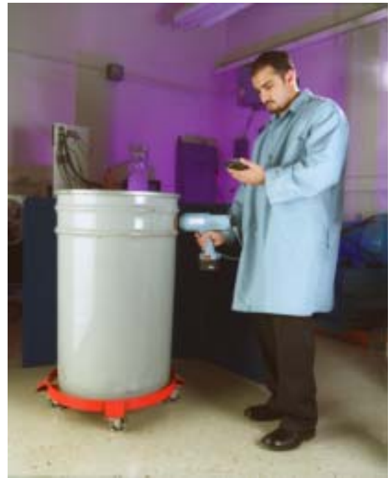
Scientists at the Pacific Northwest National Laboratory are developing an Acoustic Inspection Device that is ideal for identifying concealed objects, such as hazardous materials in closed containers.
