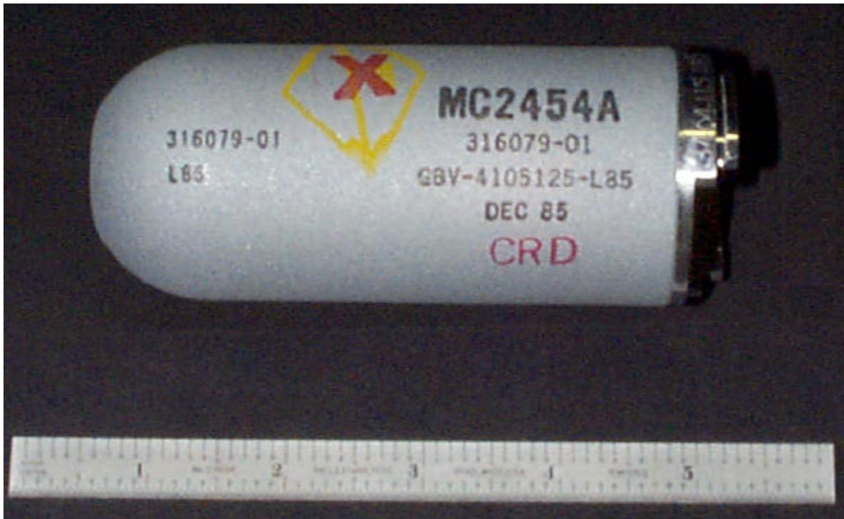
**Figure 6.1.** Unclassified Photo of a Ferroelectric Neutron Generator Tube
