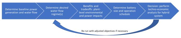
Figure 2. Energy storage sizing methodology.
