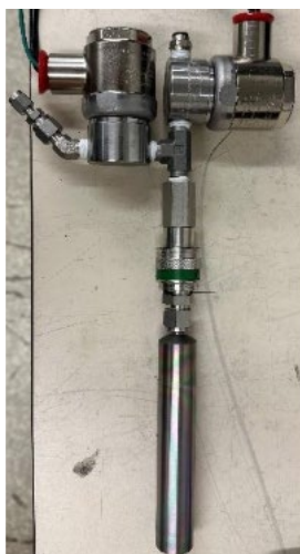
Figure 7. Sample cylinder integrated with solenoid valve assembly, illustrating automated flow control, fail-safe isolation (normally closed configuration), and regulated interaction with nitrogen carrier gas during injection and extraction.
