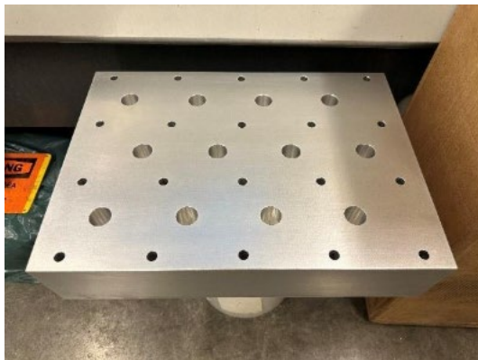
Figure 4. Precision-machined aluminum cylinder block with bored wells for nine sample and three control cylinders, designed to provide uniform heat distribution and maintain a stable thermal environment (37 °C) via embedded cartridge heaters.
