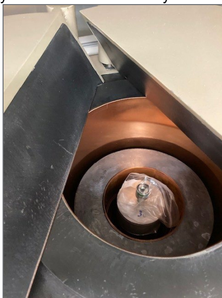
Figure 10: Sample cylinder configured for measurement on the shielded HPGe detector
