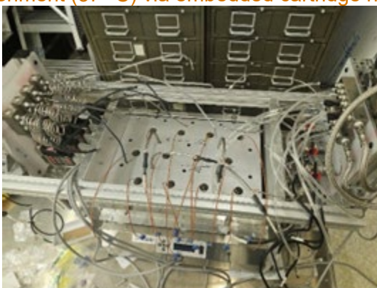
Figure 5. Installed cylinder block with integrated process tubing, thermocouples, and manifold connections, illustrating system-level routing for controlled flow distribution, temperature monitoring, and volumetrically consistent sample handling.
