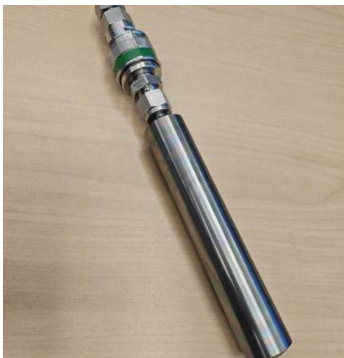
Figure 6. Stainless steel sample cylinder (60 mL total capacity) with quick-disconnect interface, designed for secure integration with the solenoid assembly, reduced analyte adhesion via electrocoating, and efficient transfer of dissolved xenon samples. Aqueous samples and controls are nominally 30 mL.
