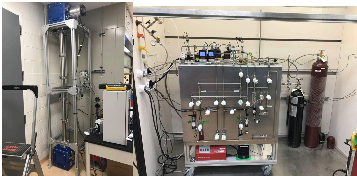
Figure 3. Photo of microchannel distillation column and system.
