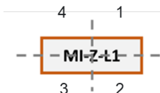
Figure 3.44. Sample cutting scheme for MI-Z-L1. Numbers 1 through 4 indicate sample number in the cutting scheme, with samples 1 and 3 shipped to PNNL, and 2 and 4 shipped to INL.
