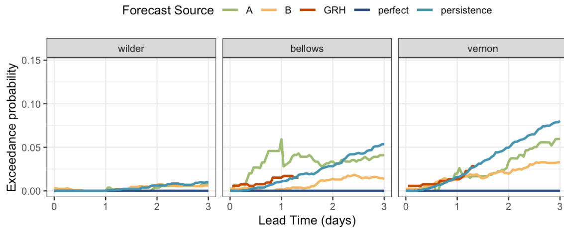
Figure 7 Probability of exceeding a 0.5 foot operating range given a neutral forebay starting position on day 0.
