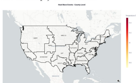
Figure 7. Examples of visualization failures observed during evaluation, including incomplete maps with missing counties, caused by JSON output truncation when result sets exceed model output limits.
