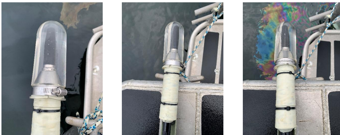
Figure 1: icListen hydrophone prior to calibration with each of the three flow shields. Flow shields 1-3 are shown from left to right. Note that the hydrophone housing was coated with white anti-biofouling paint for another project. Photos provided by Ocean Networks Canada.
