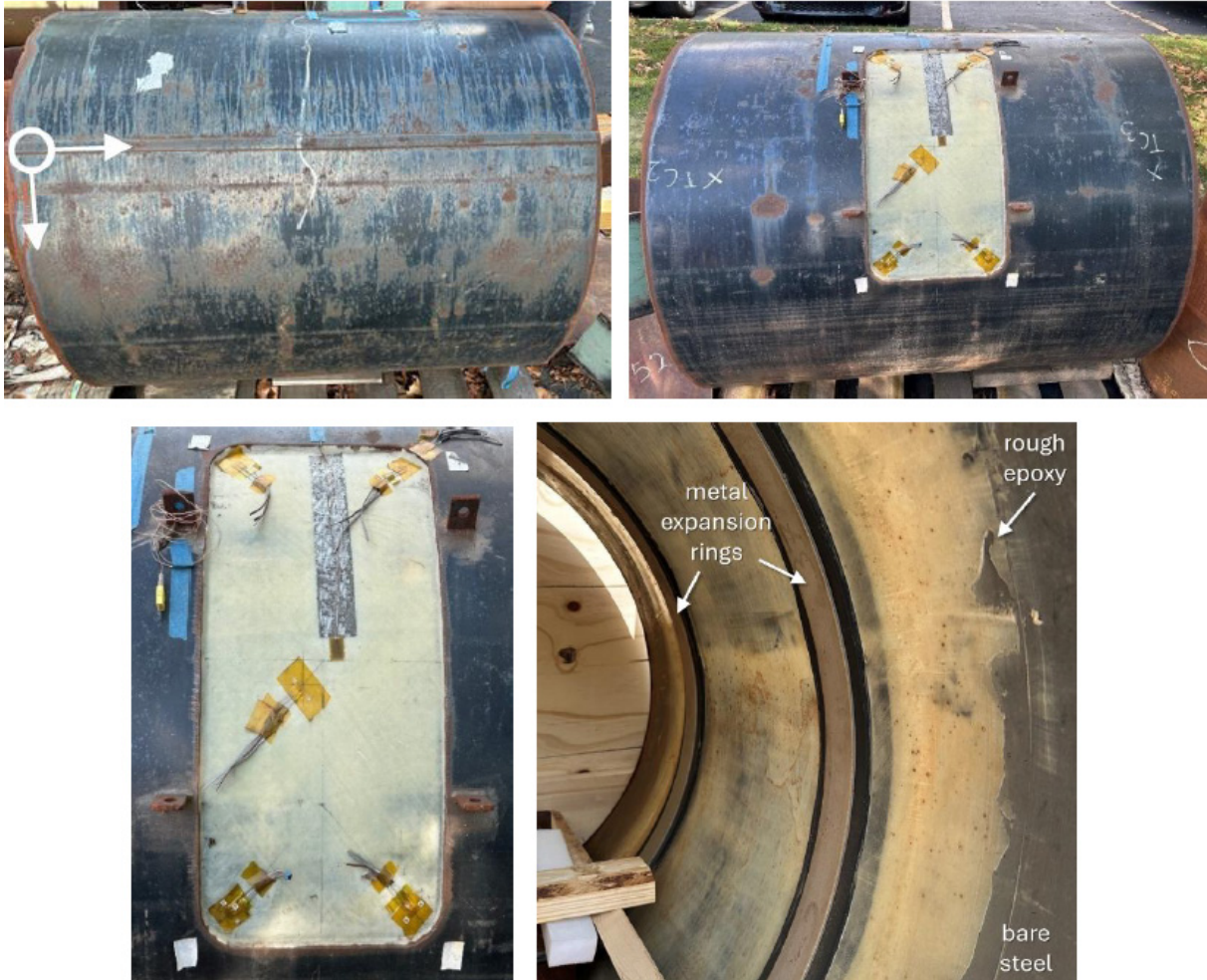
Figure 15. Photographs of the pipe mockup.
