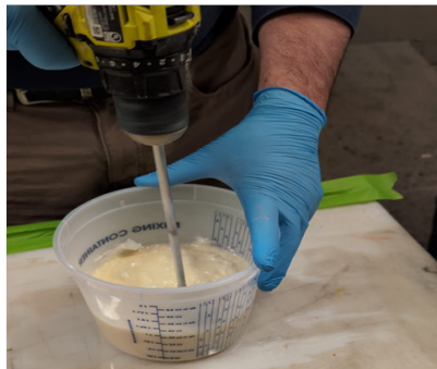
Step 3: Preparation of Putty
