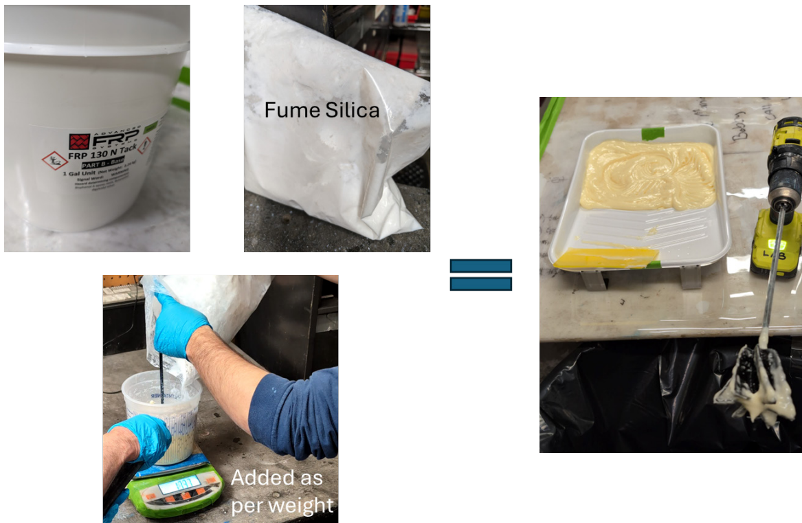
Figure A.1. Preparation of thickened epoxy.
