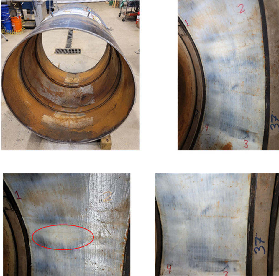
Figure 17. River-like matrix cracking on the CFRP pipe after hydrostatic testing. Images from Hioe et al. (2021).
