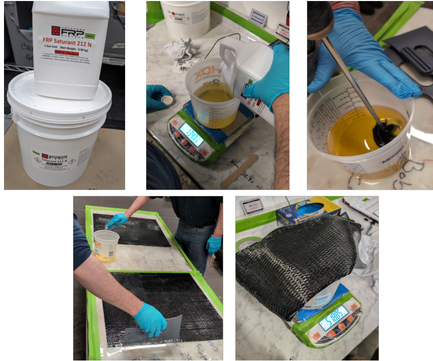
Figure A.2. Manual saturation of fabric.
