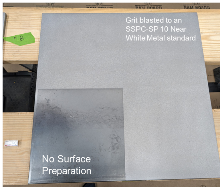
Figure 13. Surface preparation of the substrate of Mockup 8.
