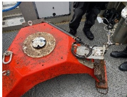
Figure 51: Biofouling on the Sea Spider on 3/24/25 at the end of Test 2.
