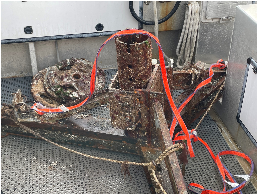
Figure 53: Biofouling on the lander when it was recovered 6/17/25.
