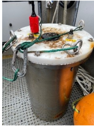
Figure 52: Biofouling on the WITT data acquisition housing on 3/24/25 at the end of Test 2.
