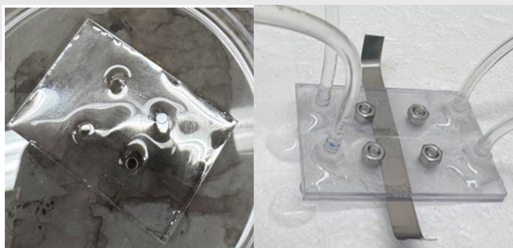
Figure 12 The Y-cell plates were coated with polyacrylamide using a spin coater (see left image). The assembled cell leaks due to potential channel blockage by the polyacrylamide coat (see right image).
