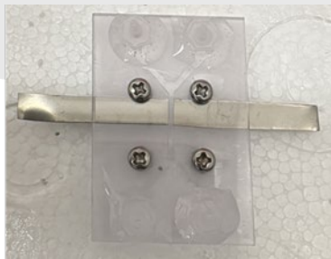
Figure 6: Example of laminar co-flow cell used for experiments using electric field.
