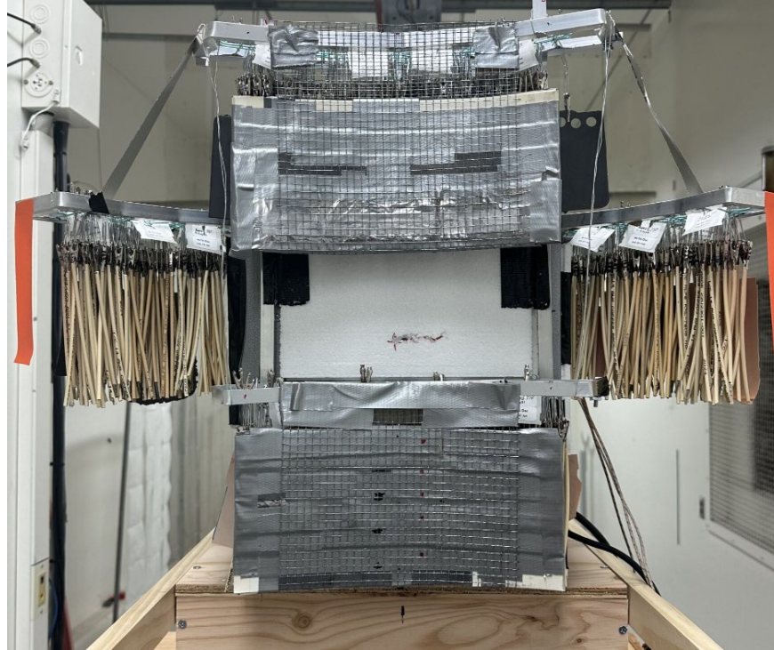
Figure 8. Arrangement of cable specimens subjected to radiation at room temperature, viewed from the side of radiation source (right view according to Figure 7a). The oven was behind the white insulation panel in the center. The lead-based beam flattening filters were added to attenuate the radiation received by cable specimens above and below the oven.
