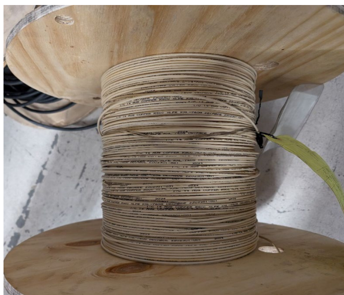
Figure 3. XLPE-dBDE cable insulation on a wooden spool.
