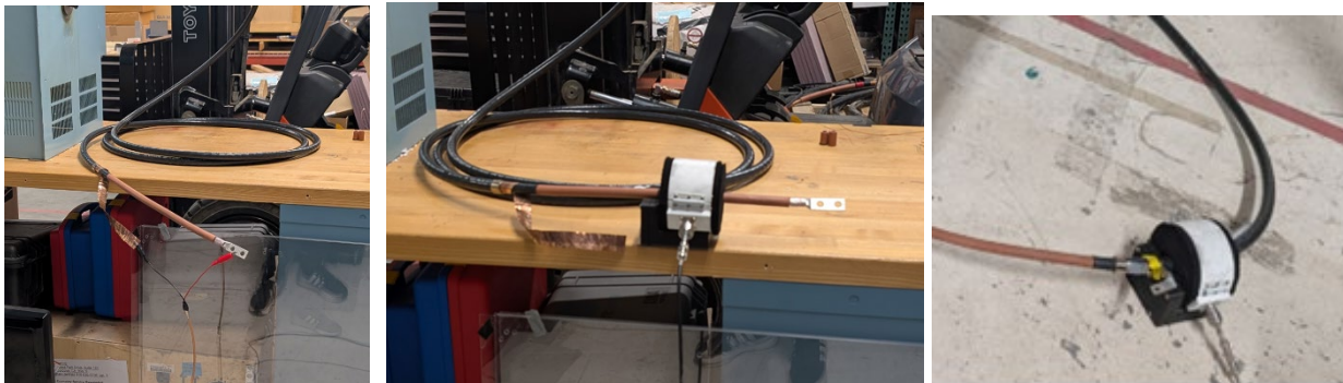
Figure 6. From left to right (a) Direct Connect (b) Iso-Coupler (c) Iso-Coupler on outer jacket.
