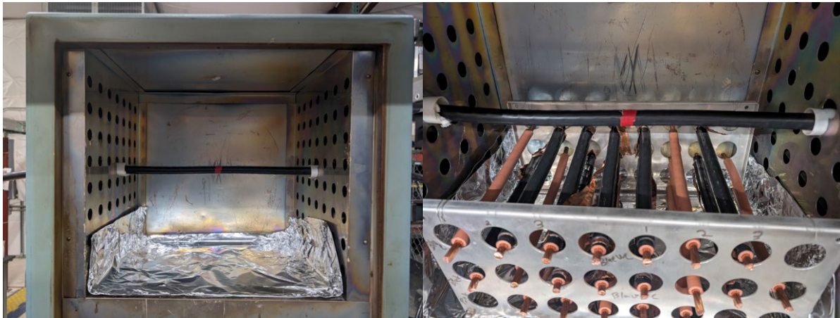
Figure 7. 4 ft segment of a 50 ft cable, in a thermal aging oven with the witness samples.
