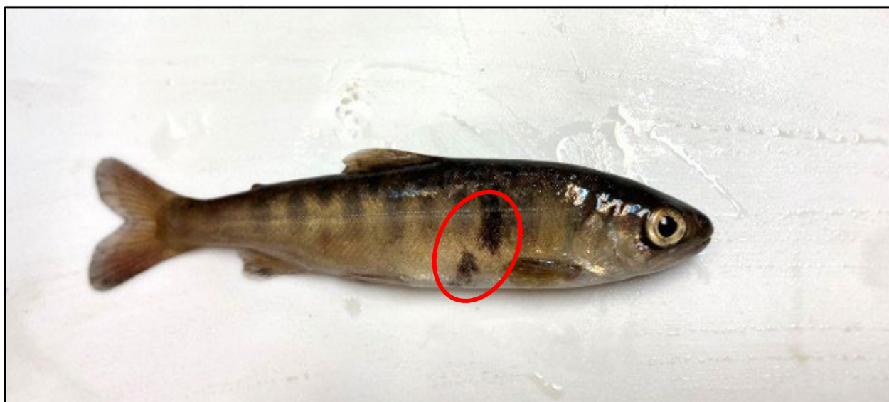
Figure 2-30. Injuries (bruising) seen on a coho salmon that did not survive exposure to a 20° plate angle at 50 fps.
