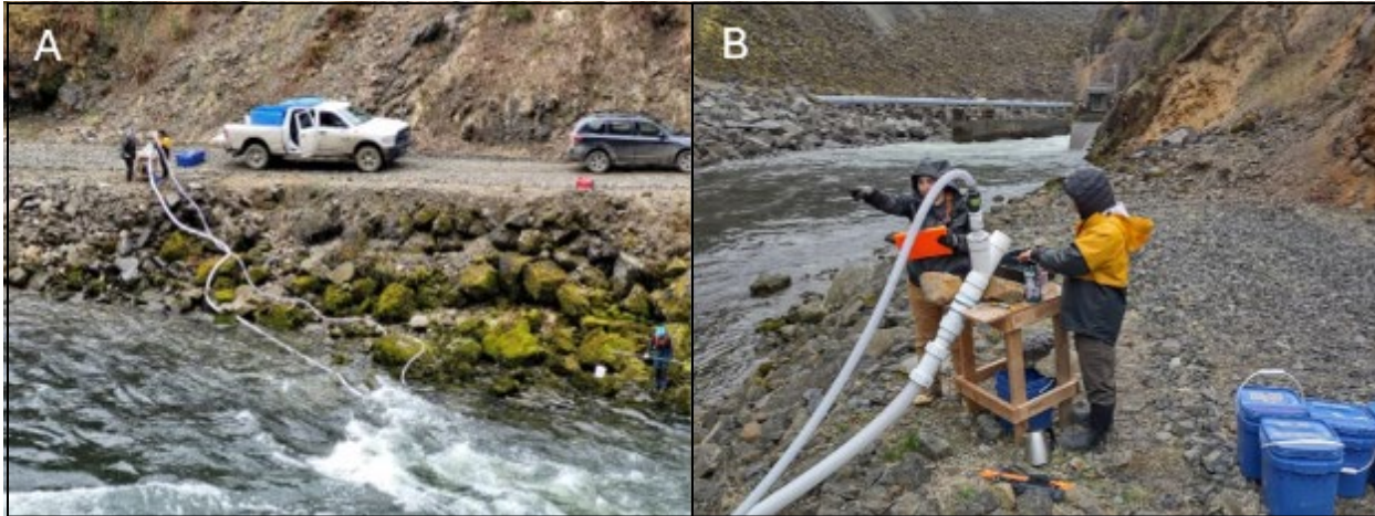
Figure 4-2. The control release system at HAHD. (A) View from the east bank of the Green River, showing the wider white release hose (left) and the white hose connected to a submersible pump (right) that flushes water through the release hose. (B) Close-up view of the system, with the flex hose attached to the top of the PVC Y-piece linked to the submersible pump and the release hose attached to the bottom for water flow.
