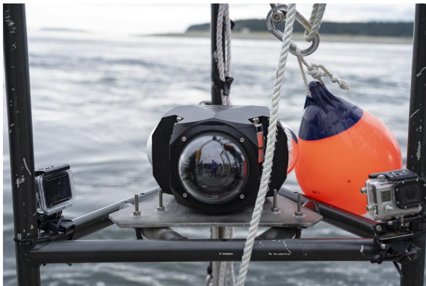
Figure 5: The Boxfish-360 camera mounted securely on the lander before deployment. GoPro's were mounted to the lander as well to collect timelapse photographs in case of Boxfish-360 malfunction.
