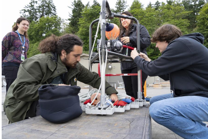
Figure 4: Team members ensuring the Boxfish-360 camera is securely attached to the weighted lander and the camera settings are adjusted to the correct format.
