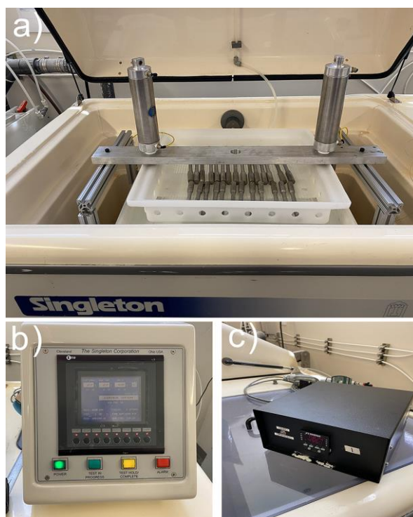
Figure 3: Photographs illustrating the SCC setup placed within the modified Singleton environmental chamber. a) Plastic sample tray (with holes on the side walls) and pneumatic actuation mechanism to move the samples in and out of the salt solution at periodic intervals. b) Singleton controller showing the current temperature of the container. c) Controller box with a counter to record the number of immersion + drying cycles during the test duration.
