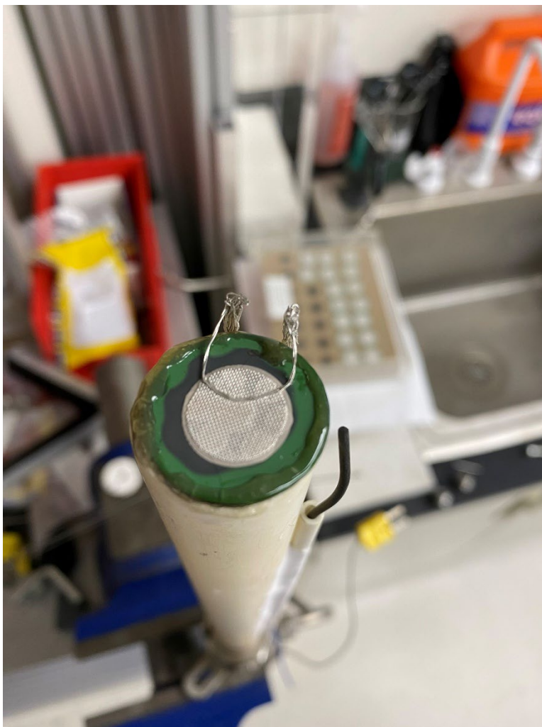
Figure 5. Four-layer GDC cell after testing.
