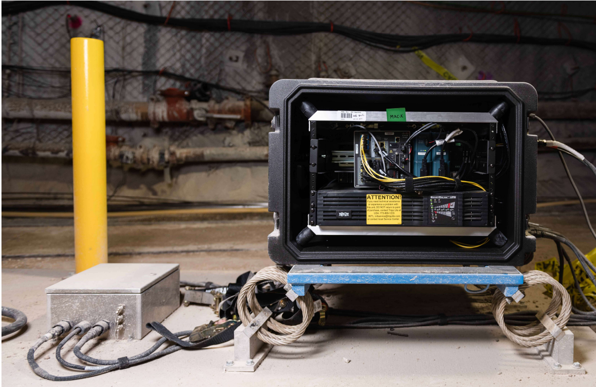
Figure 21 Photos illustrating the level of dust reduction for the interior of IDAQ nodes relative to the environmental conditions outside
