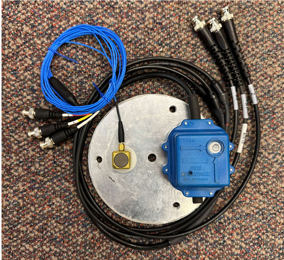
Figure 15 IDAQ ground motion sensors and mounting disk
