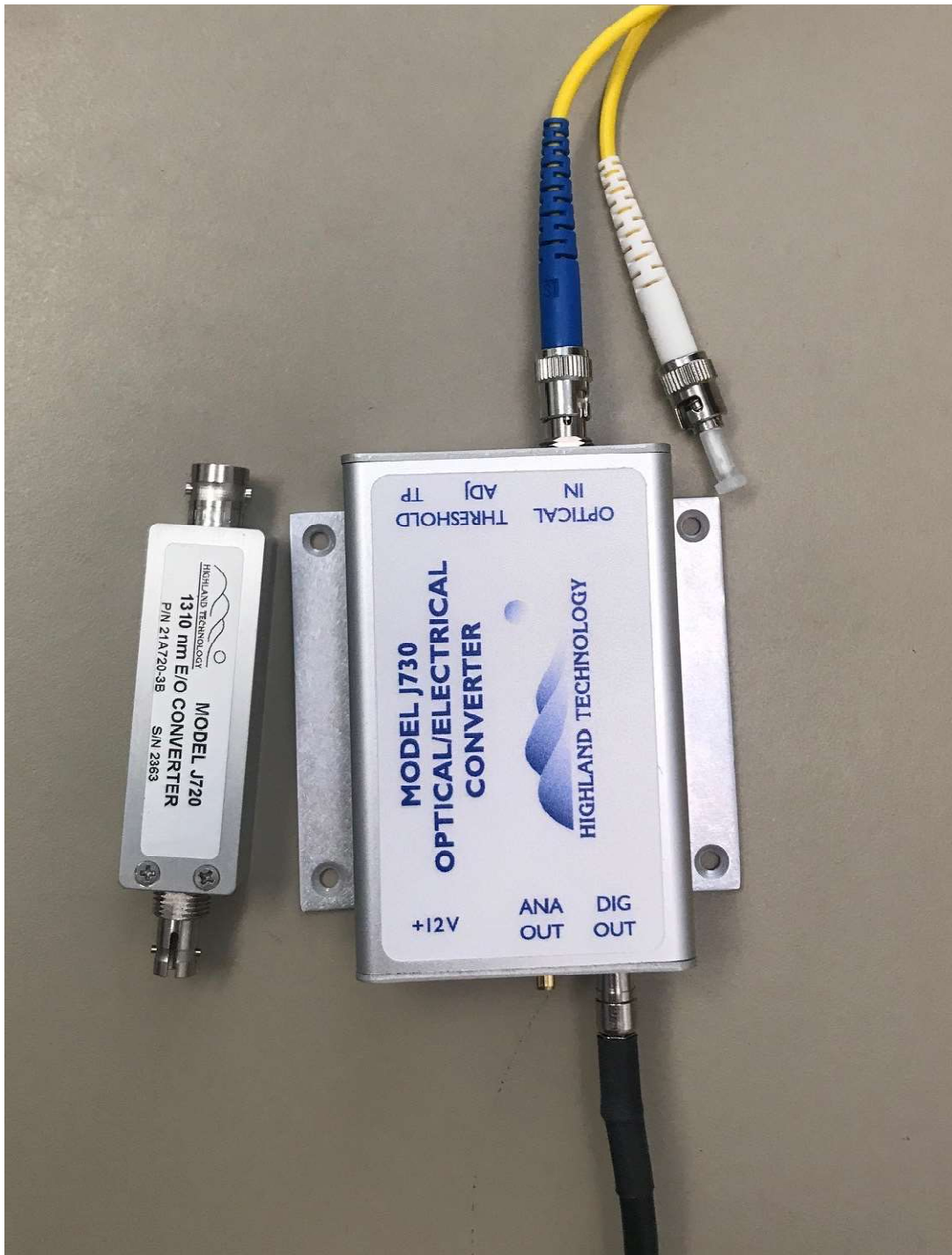
Figure 9 Electrical to optical and optical to electrical converters used for the PE1 IDAQ trigger distribution network
