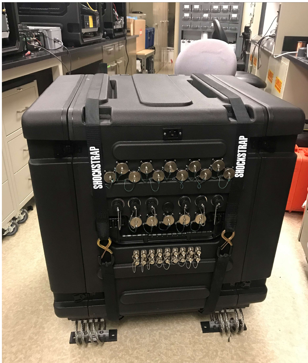
Figure 10 SRS distribution amplifier used for trigger relay at the P.06 bypass drift 650 facility
