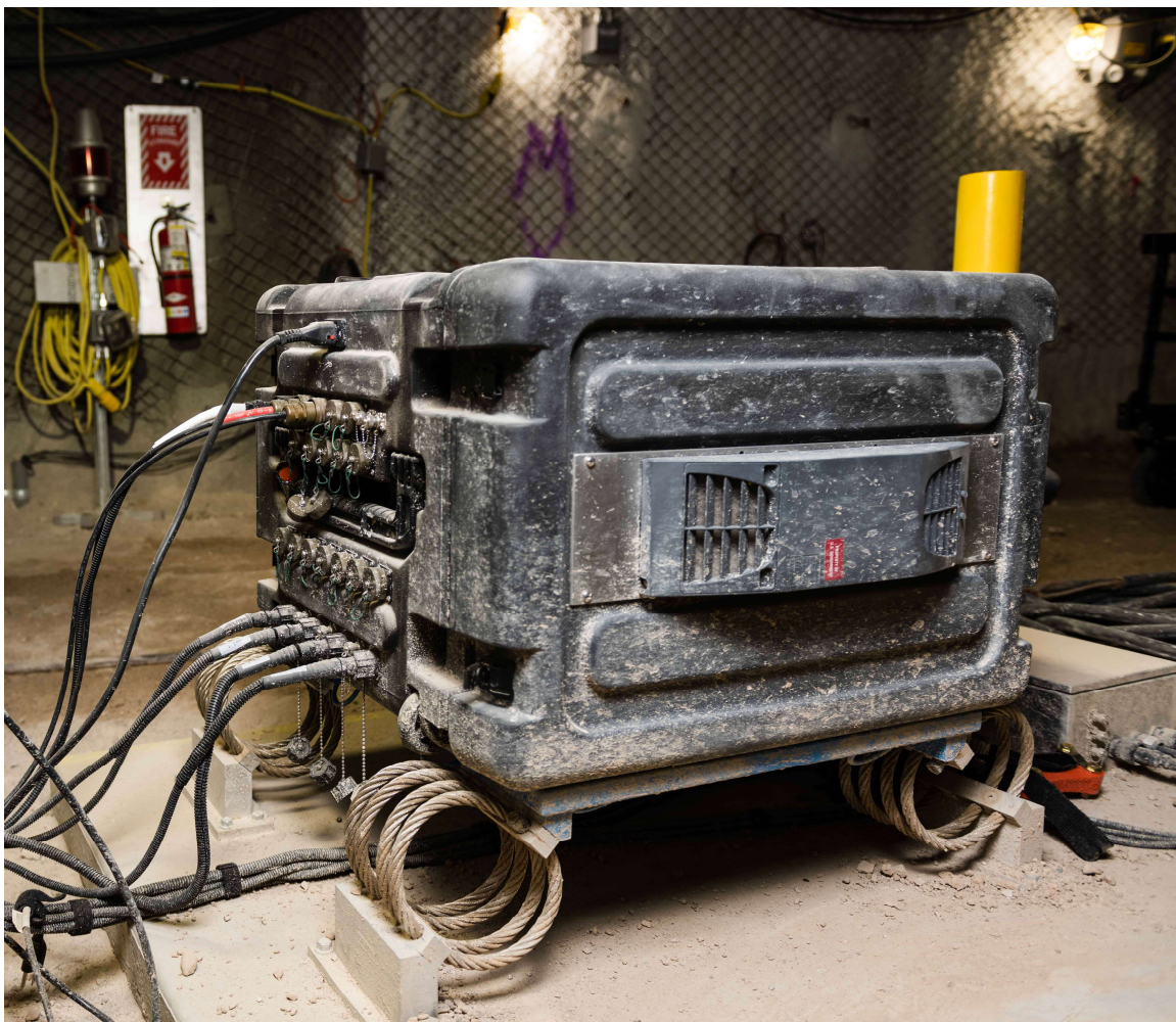
Figure 5 IDAQ node at MAC-Y location illustrating features used to protect from harsh underground environments
