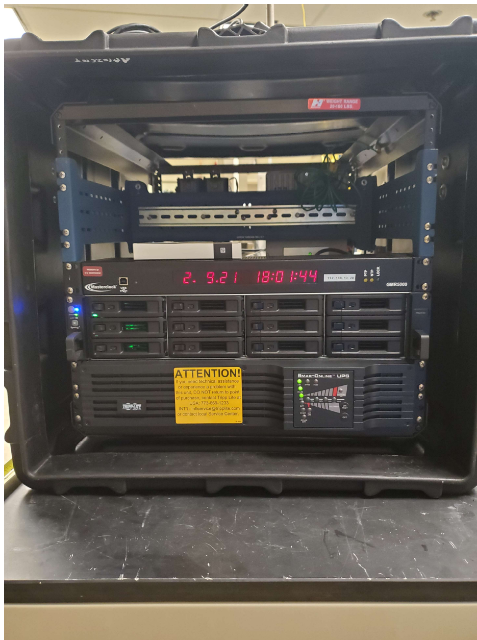
Figure 11 IDAQ ARMAG1 node containing master clock, RAID drive, and UPS
