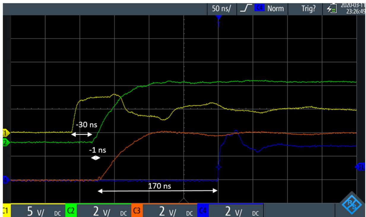
Figure 20 Test signals: Yellow is PPS signal from IDAQ clock; green is PPS signal from HE T&F clock; red is pulse out of the HE T&F clock-trigger; blue is the trigger received at the IDAQ NI-9402
