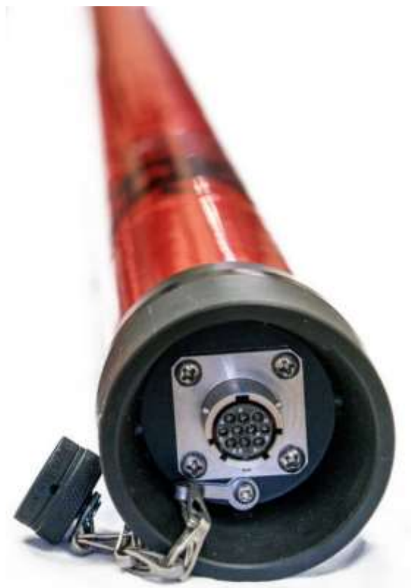
Figure 18 Low frequency electromagnetic B-field, Phoenix Geophysics model MTC-150, sensor recorded by the 1010 IDAQ node
