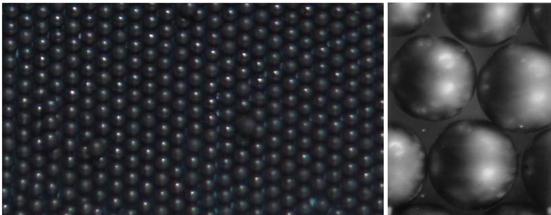
Figure A-4. Sintered UO 2 Kernels of 500–532 μm Diameter (Collins et al. 2004).
